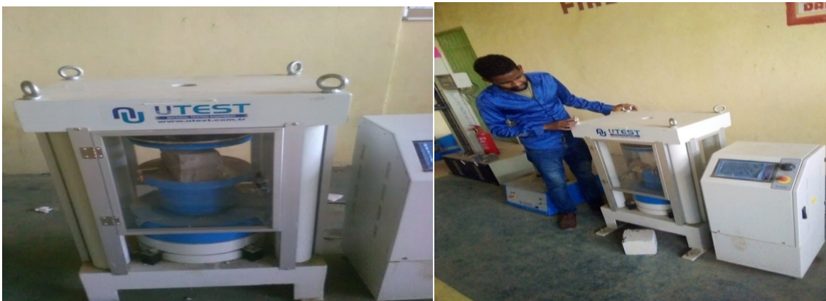
Figure 3.13: Compression strength test on brick to determine the load carrying capacity of bricks under compression (4/14/2021)
