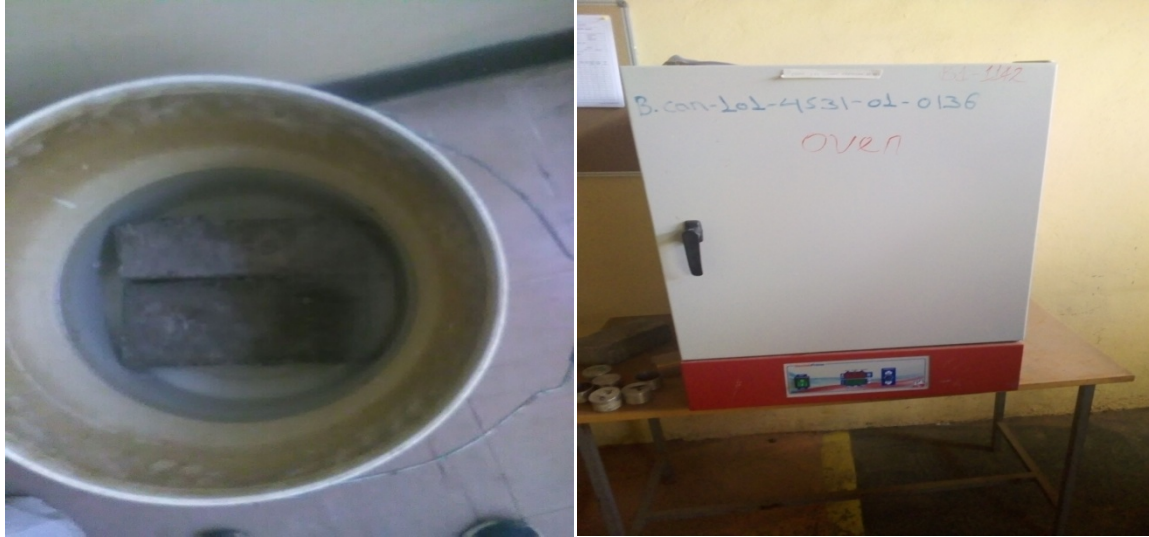
Bricks immersed in to water and dried in oven dry (photo taken by me)
