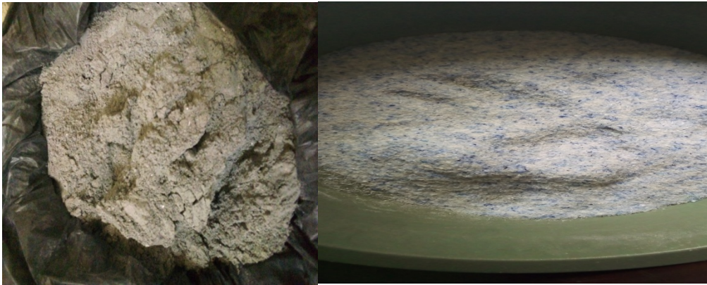
Shredding and cutting of PET and fly ash (Photo taken by me)
