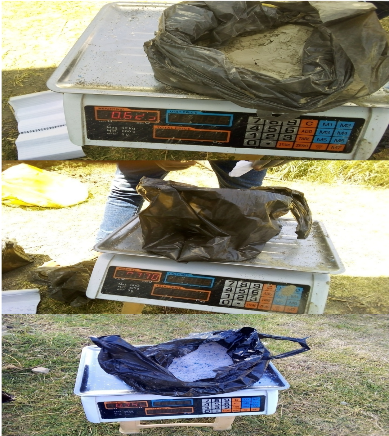
Weighing or Batching of PET plastic waste, cement, Flyash and sand( photo taken by Belete Asegdew)
