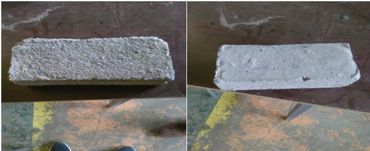
Figure 3.11: Plastic fly ash Brick after removing it from the mould (14/4/2021)
