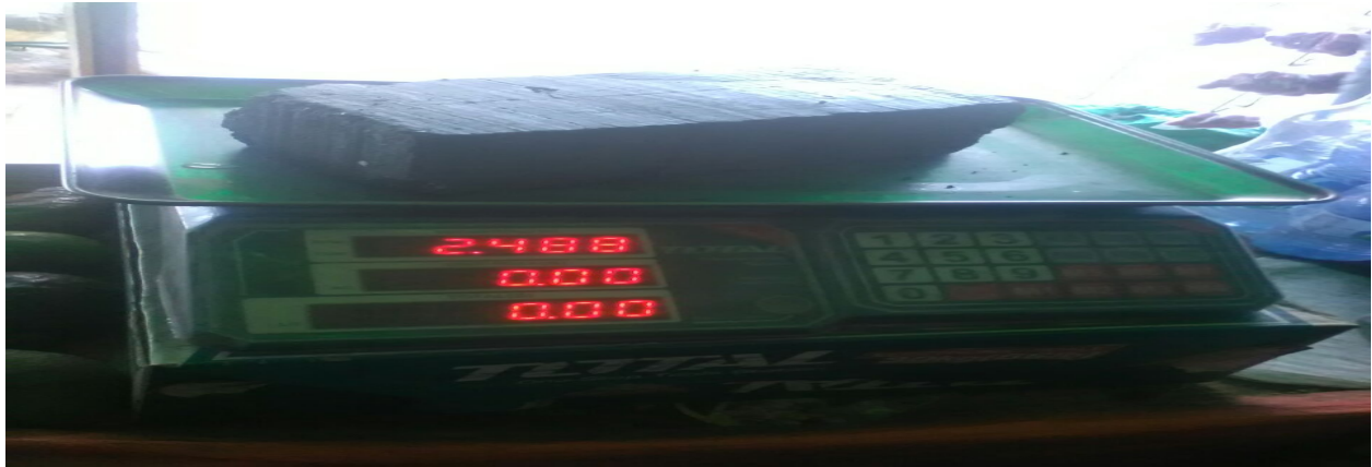
Weighing of bricks (photo taken by me)
