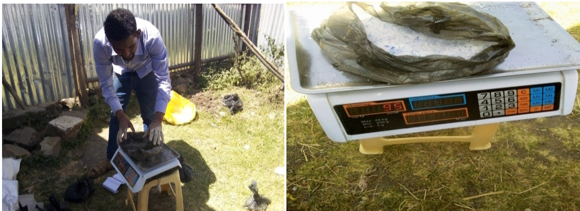
Figure 3.8: Batching (Measuring) of plastic waste, fly ash, cement and sand (3/14/2021)
