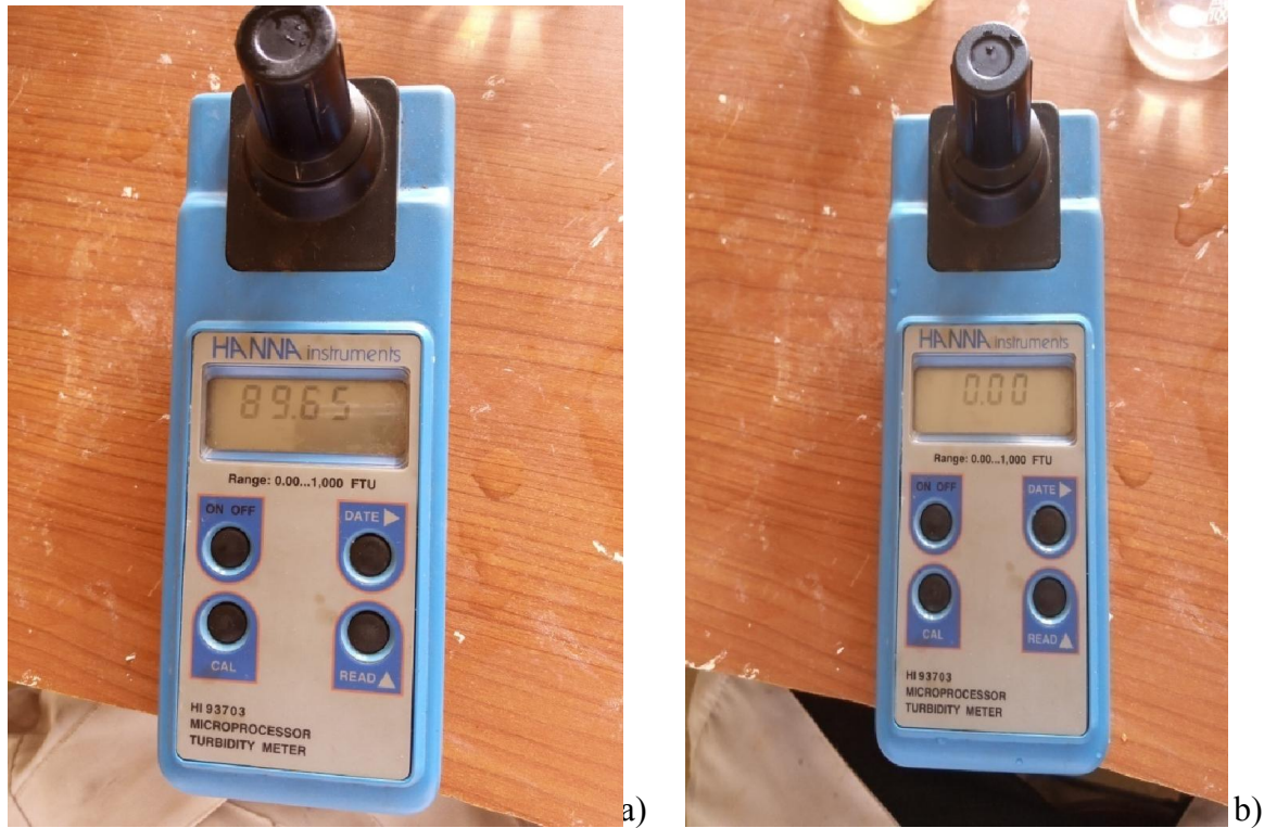
Figure 3.6 Turbidity measurement of the sample a) before treatment and b) after treatment
