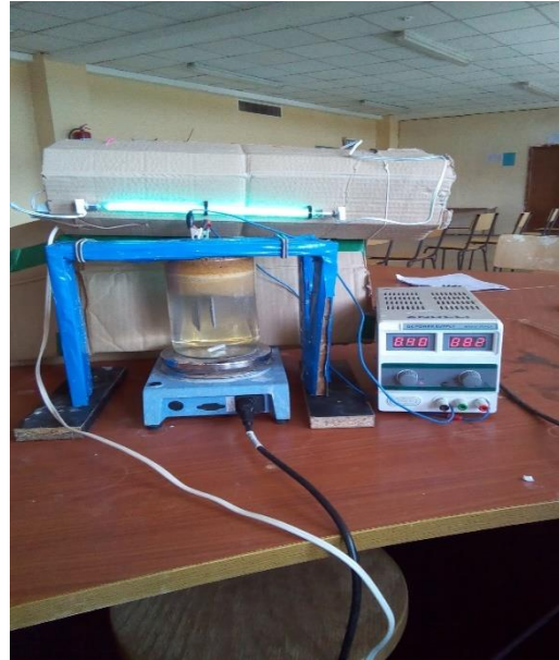
Figure G-3 Adjusting variables and treatment by using combination of UV/H 2 O 2
