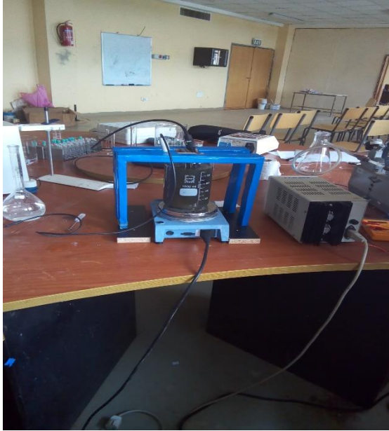
Figure G-3 Adjusting variables and treatment by using combination of UV/H 2 O 2
