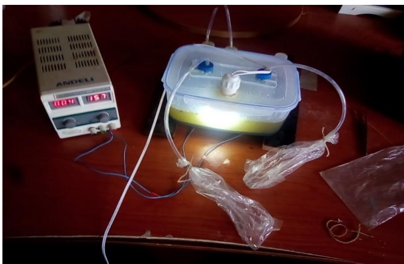
b) Plastic bags connected with gas tubes
