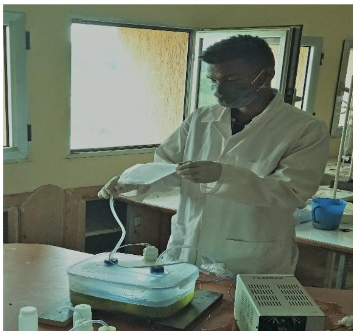
d) Separate the plastic from the gas tube safely when the required time is reached
