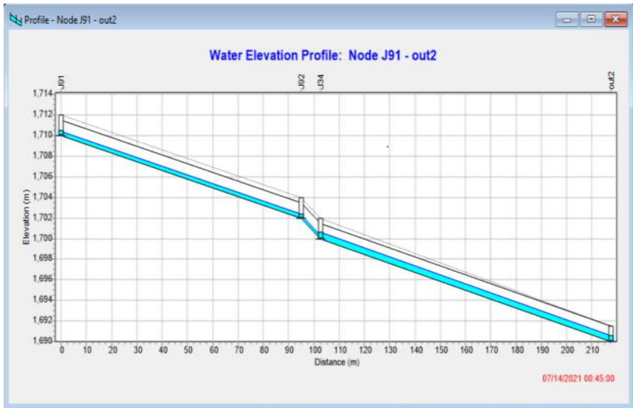
Figure 4.10: Water elevation profile around outlet-2
