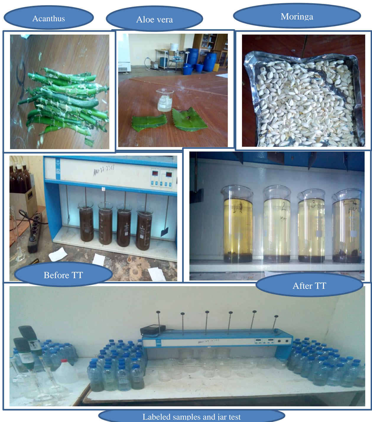
Figure 3.1: Photographic representation of WCPWW treatment using wet AS, moringa, aloe vera and blended form coagulants.
