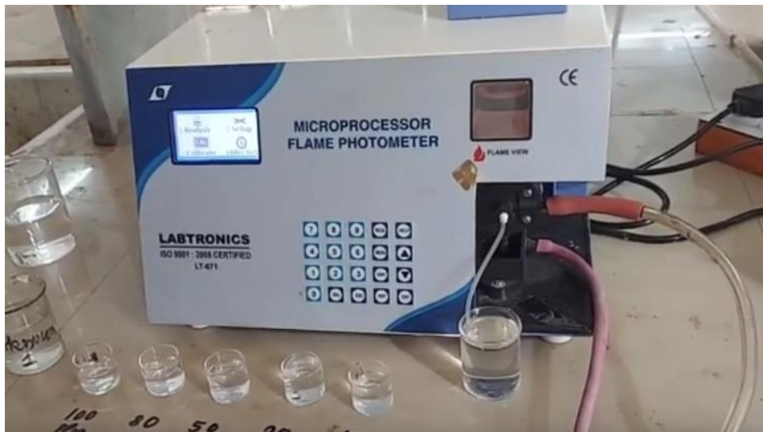
Figure 9 During conducted of the experiment potassium in the Microprocessor Flame photometer chemistry lab WKU.
