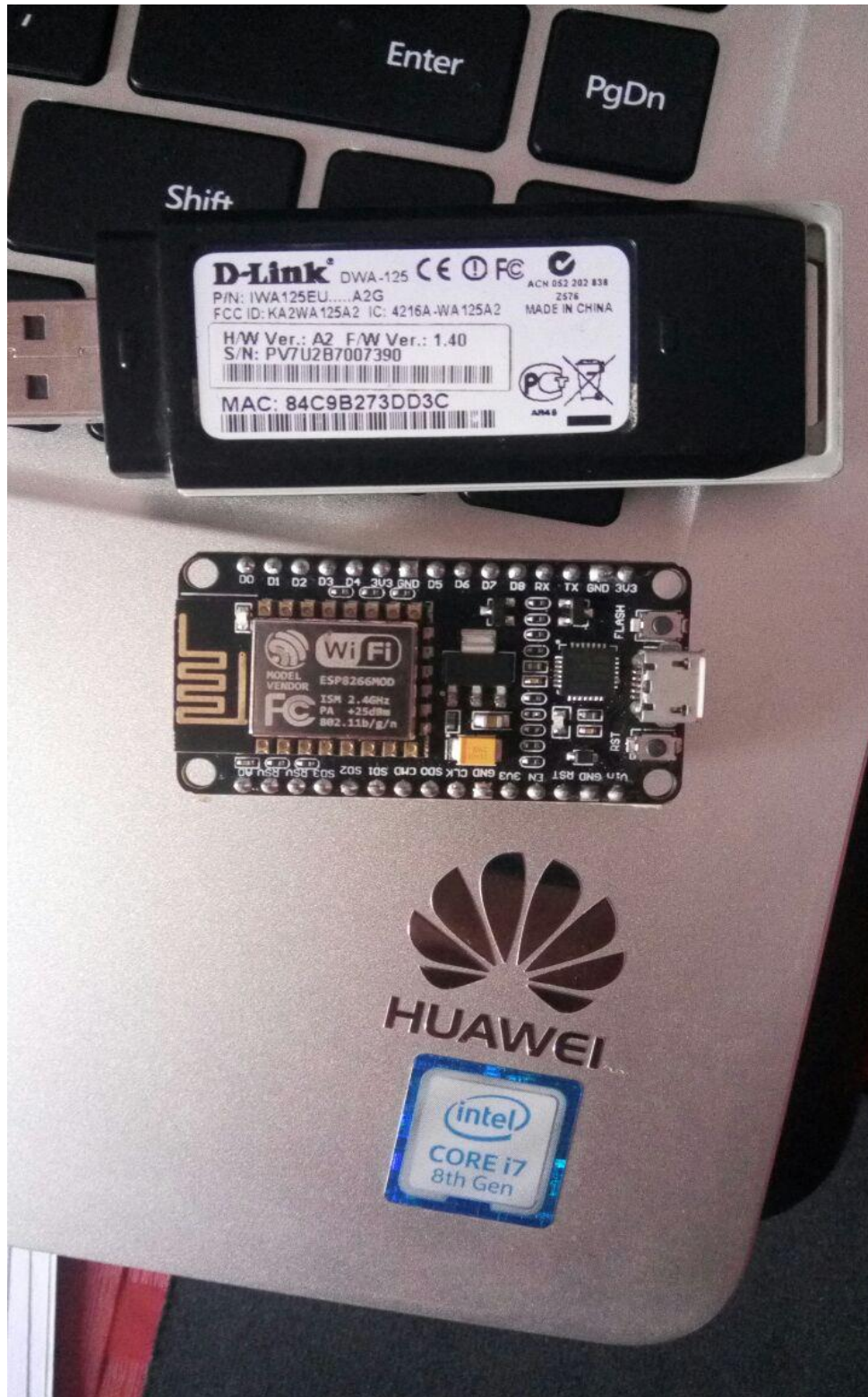
Fig 3: NodeMCU and D-Link DWA
