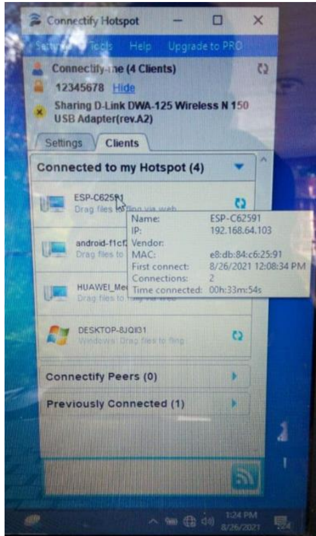
Fig 4: IP and MAC address of NodeMCU
