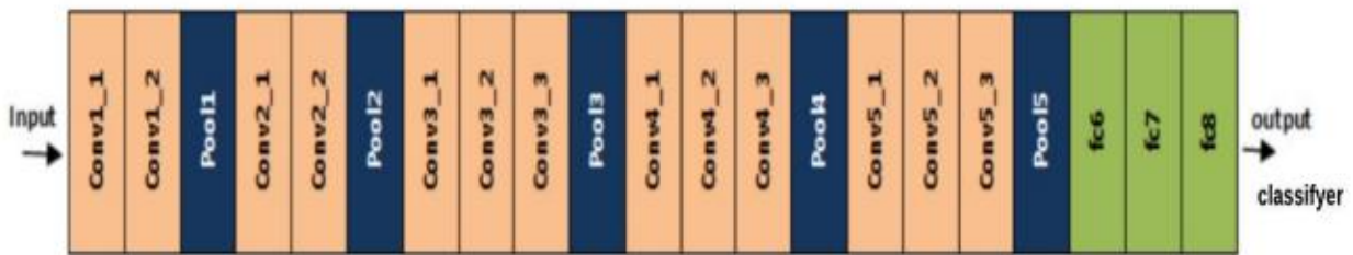
Figure 2. 20 The Architecture of VGGNet [73]
