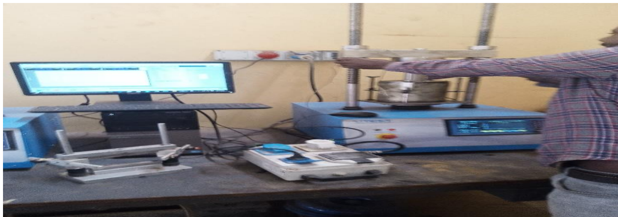
Figure 3-5 Photo during the Determination of California bearing ratio test (June 16 2021 Captured by Euel)
