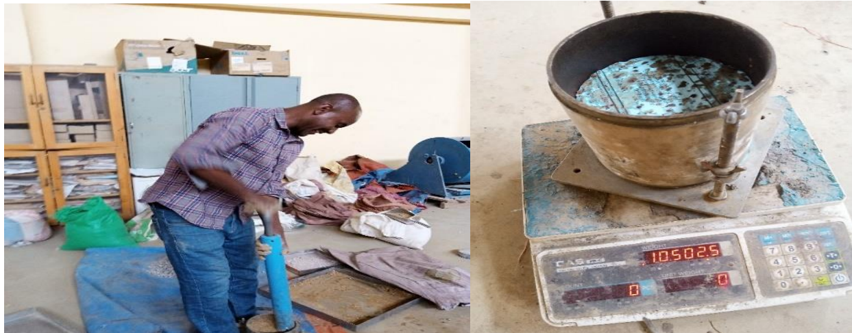
Figure 3-4 Photo during the Determination of Compaction test (June 12, 2021, Captured by Biniyam
