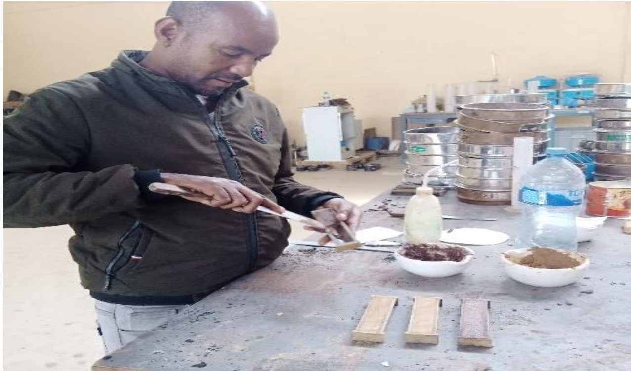
Figure 3-6 Photo during the Determination of Shrinkage limit (July 01 2021, Captured by Haile)
