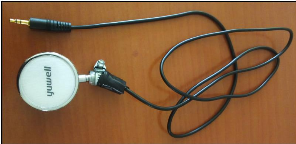
Figure 4.8: SG electret microphone connected to head of traditional stethoscope and an audio cable.
