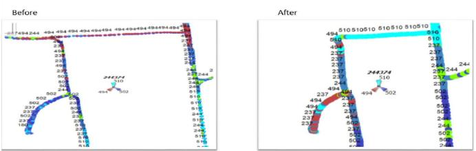
Problem: All of three sectors of 244374 CPRI Cable of DUW Mismatch installed Solution: Exchange CPRI Cable of Sector C to Sector A , Sector A to Sector B ,Sector B to Sector 3 Observation: The Three crossed sector serves it's own coverage area After Exchanging CPRI Cable from DUW for the
