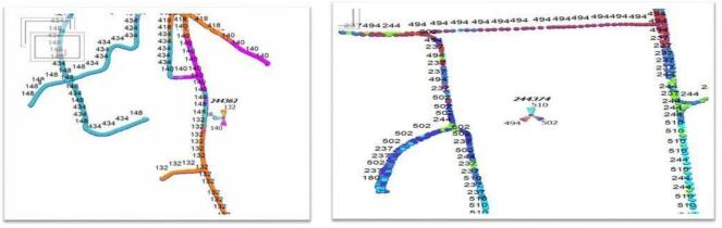
Problem: Sector A (SC 132) CPRI Cable of DUW & Sector C (SC140) CPRI Cable of DUW Mismatch installed Solution: Exchange CPRI Cable of Sector A to Sector C & Sector C to Sector A & Retest
