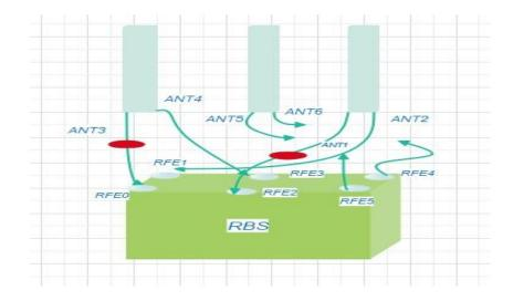
Figure 3. 7. Crossed Antenna Connection
