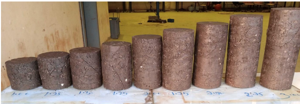
3.5. Failure patterns of 100mm diameter specimens JiT Campus test pit
