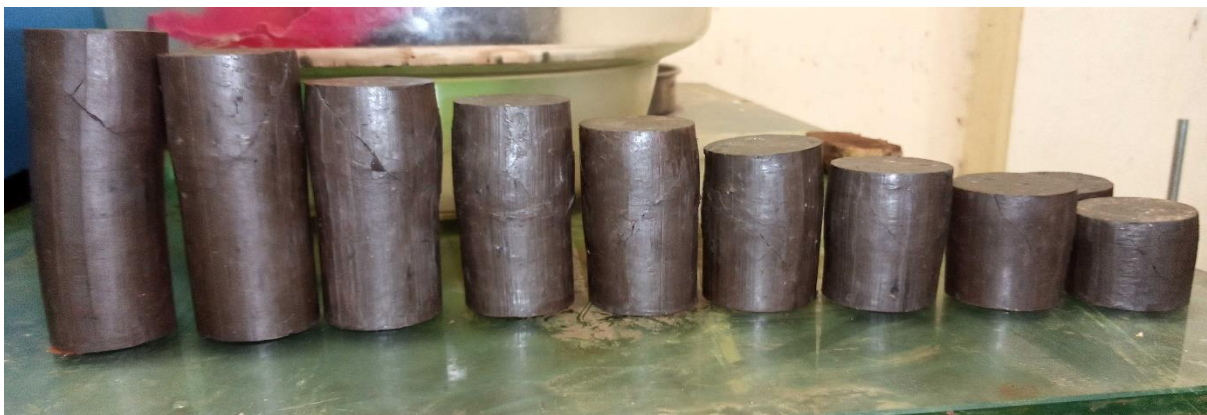
1.5. Failure patterns of 38mm diameter specimens JiT Campus test pit
