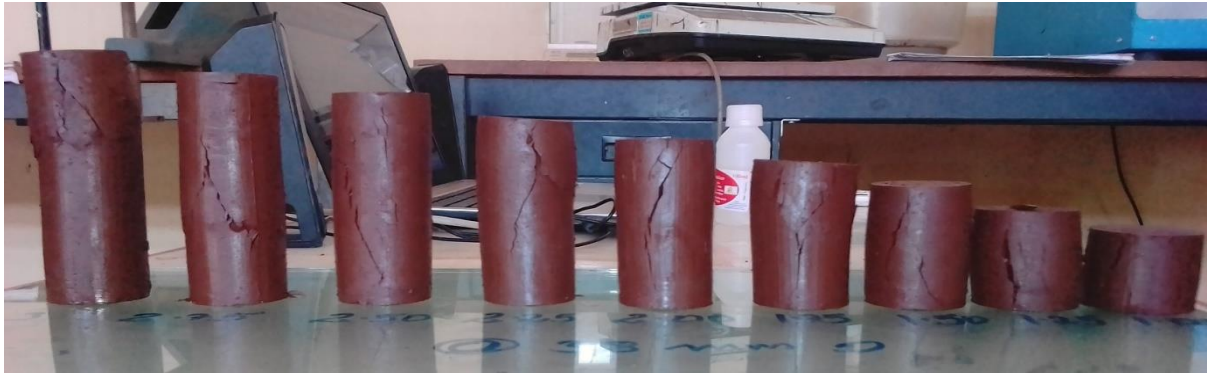
1.4. Failure patterns of 38mm diameter specimens Saris Sefer test pit
