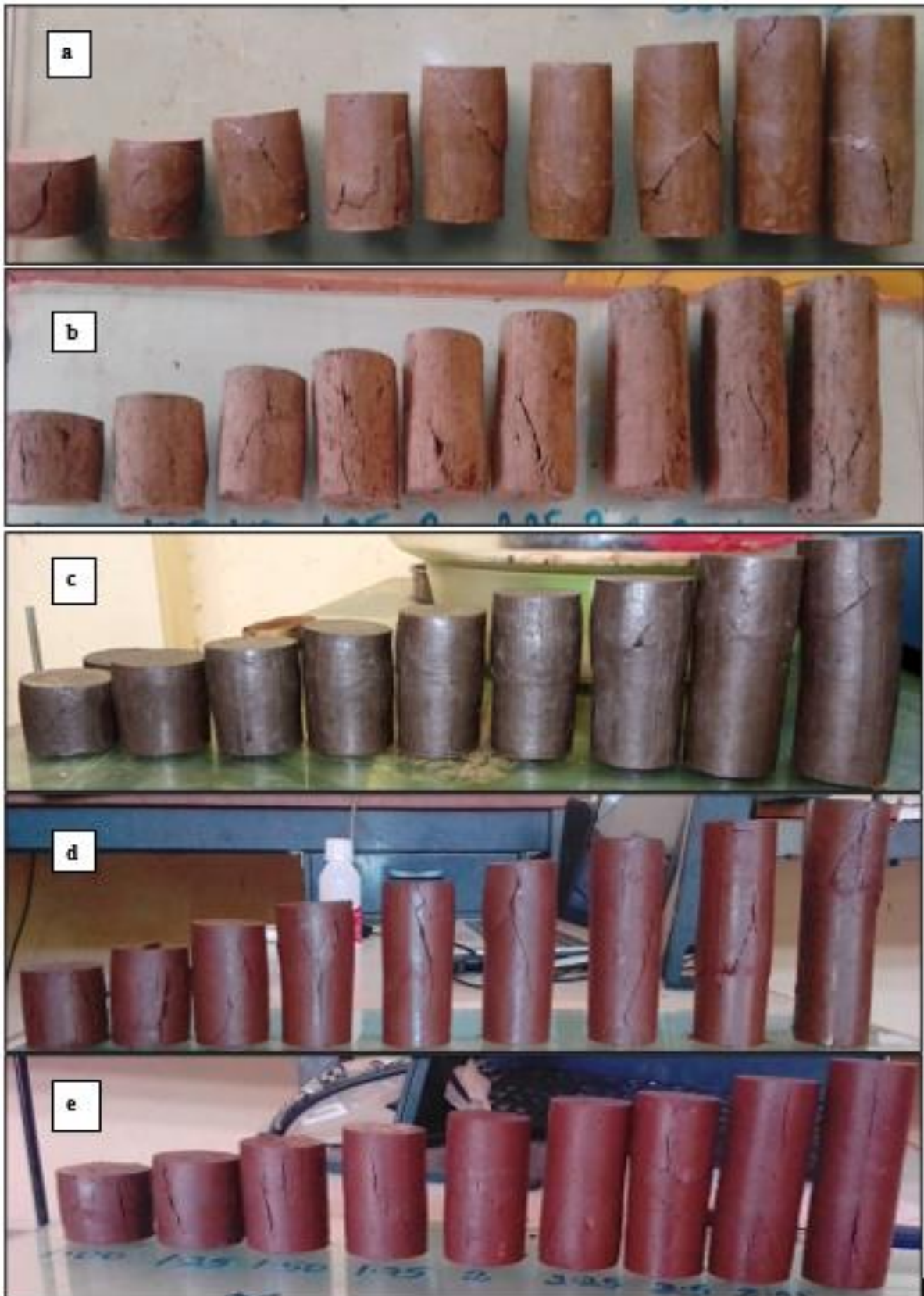
Figure 4-8 Failure pattern of 38mm specimen diameter, a- Ajip, b- Aweytu, c- JiT Campus, d- Saris Sefer and e- Mariam Church
