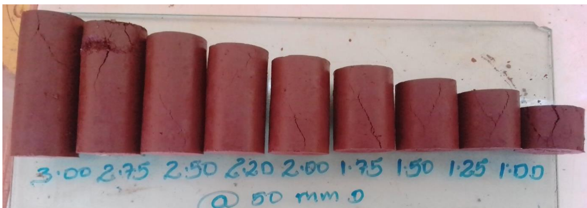
2.4. Failure patterns of 50mm diameter specimens Saris Sefer test pit
