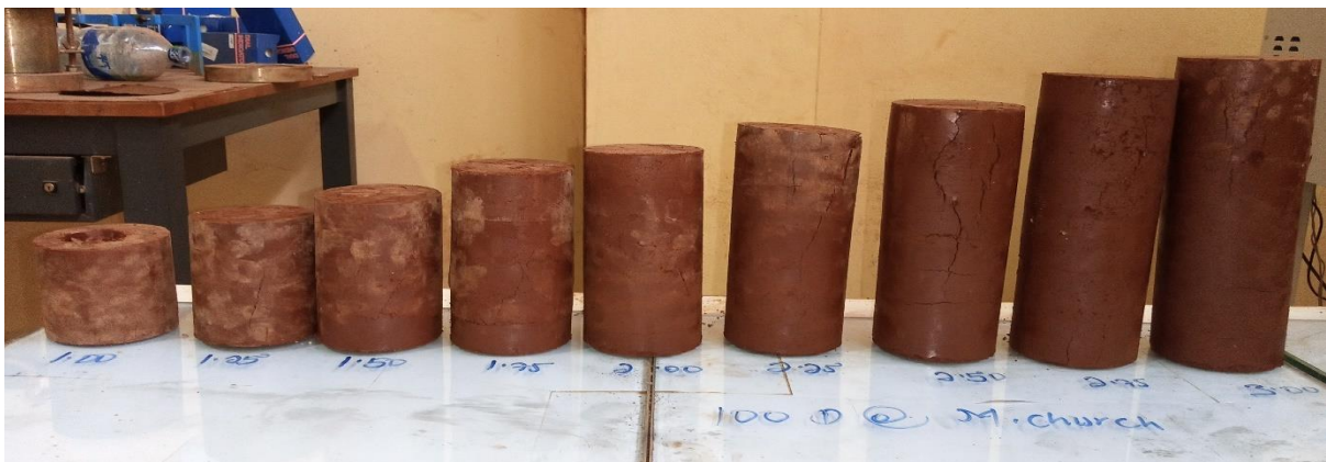
3.1. Failure patterns of 100mm diameter specimens Mariam church test pit
