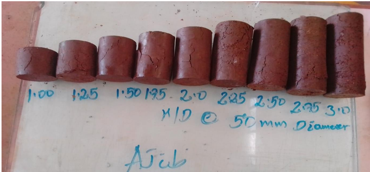
2.2. Failure patterns of 50mm diameter specimens Ajip test pit
