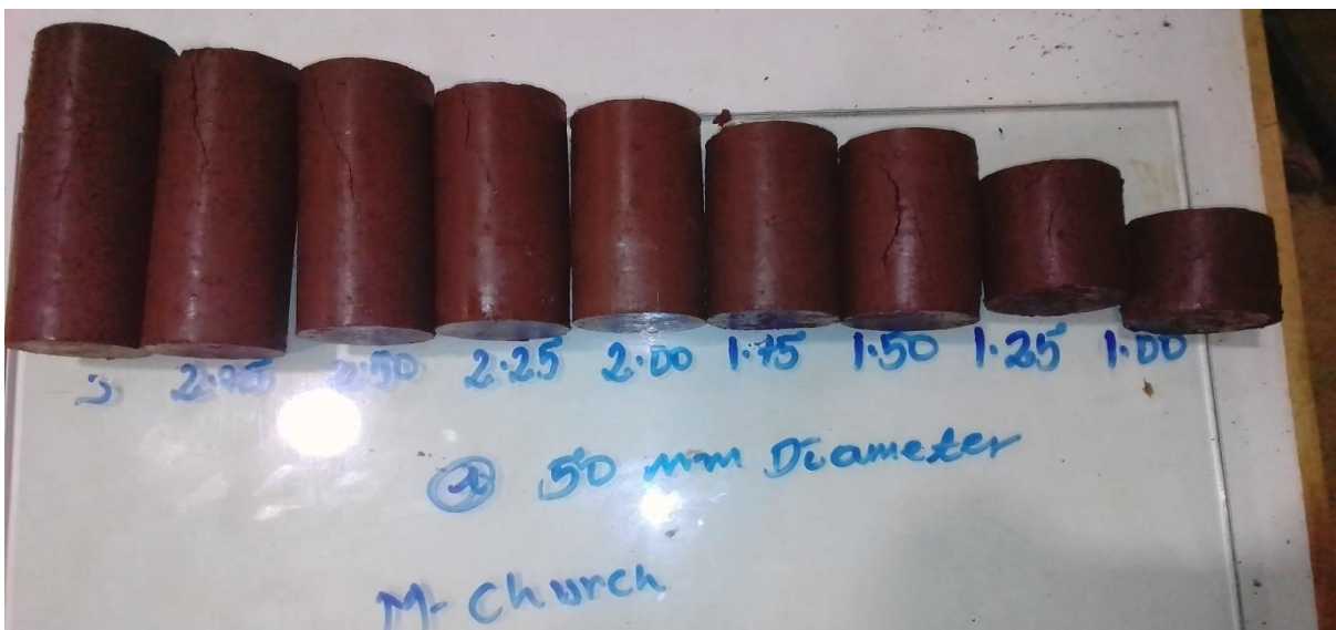
2.1. Failure patterns of 50mm diameter specimens Mariam church test pit
