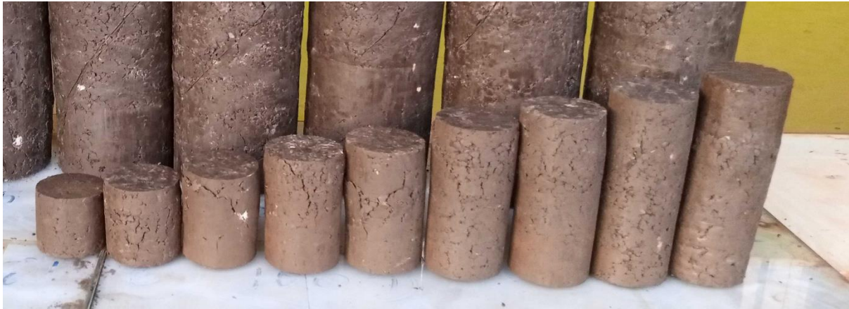
2.5. Failure patterns of 50mm diameter specimens JiT Campus test pit
