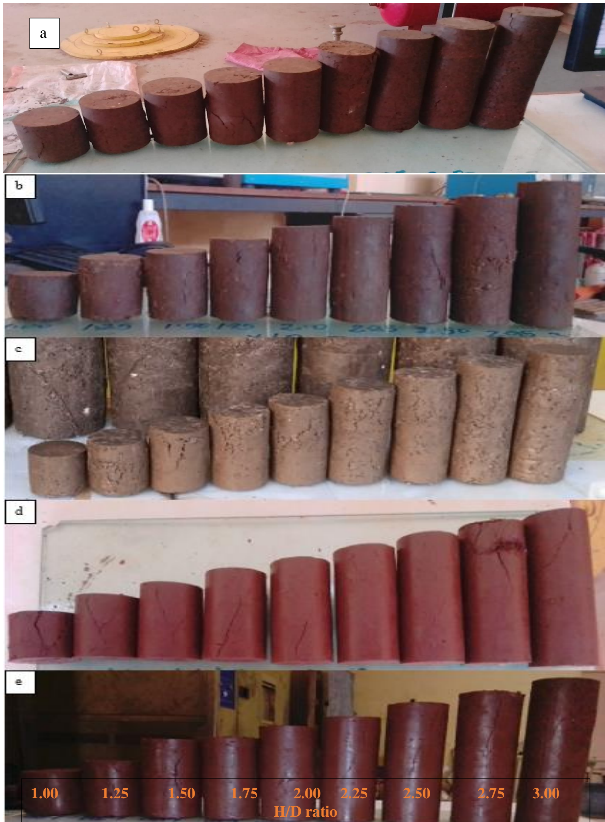
Figure 4-9 Failure pattern of 50mm specimen diameter, a- Ajip, b- Aweytu, c- JiT Campus, d- Saris Sefer and e- Mariam Church
