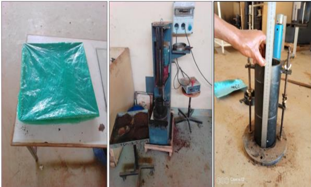
Figure 3-3 Preparation of Compacting Cohesive Soil Specimen for Unconfined Compression Test
