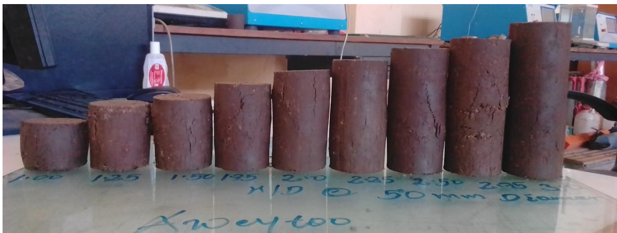
2.3. Failure patterns of 50mm diameter specimens Aweytoo test pit
