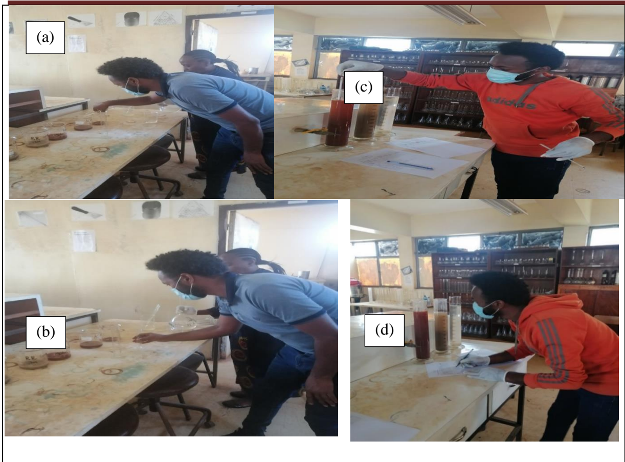
Figure 7: Determination hydrometer tests (photo captured by Adisalem G.) (a) sample preparation and add dispersing agent (b) mixing the soil sample with dispersing agent by using string (c) insert the thermometer into glass jar and d) recording the data
