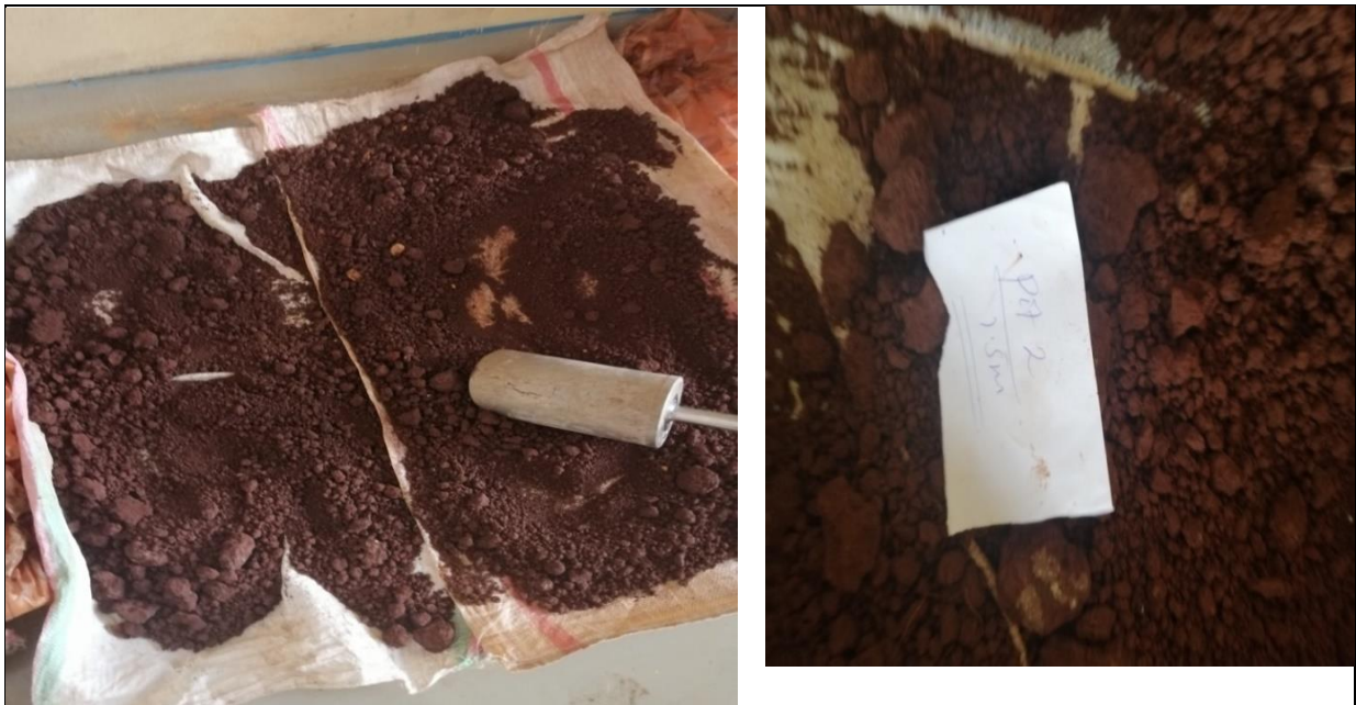
Figure 2: Disturbed sample preparation procedure
