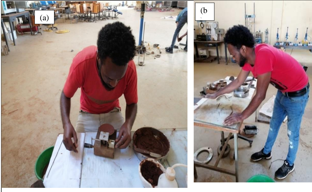
Figure 5: Determination Atterberg's limit tests (a) liquid limit using Casagrande apparatus (b) plastic limit using plastic method (photo captured by Adisalem G.)
