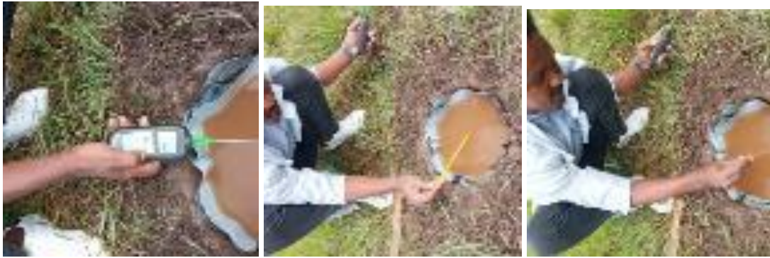
Figure 7. Measuring water temperature at surface, middle and top of pool water
