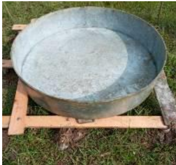
Figure 8. Setting class, A pan in the field (Jimma meteorological station)
