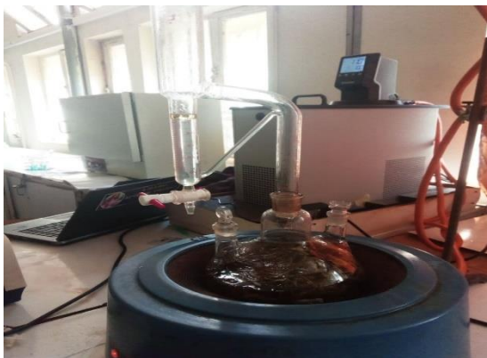
Figure 9: Hydro-distillation extraction of the essential oils
