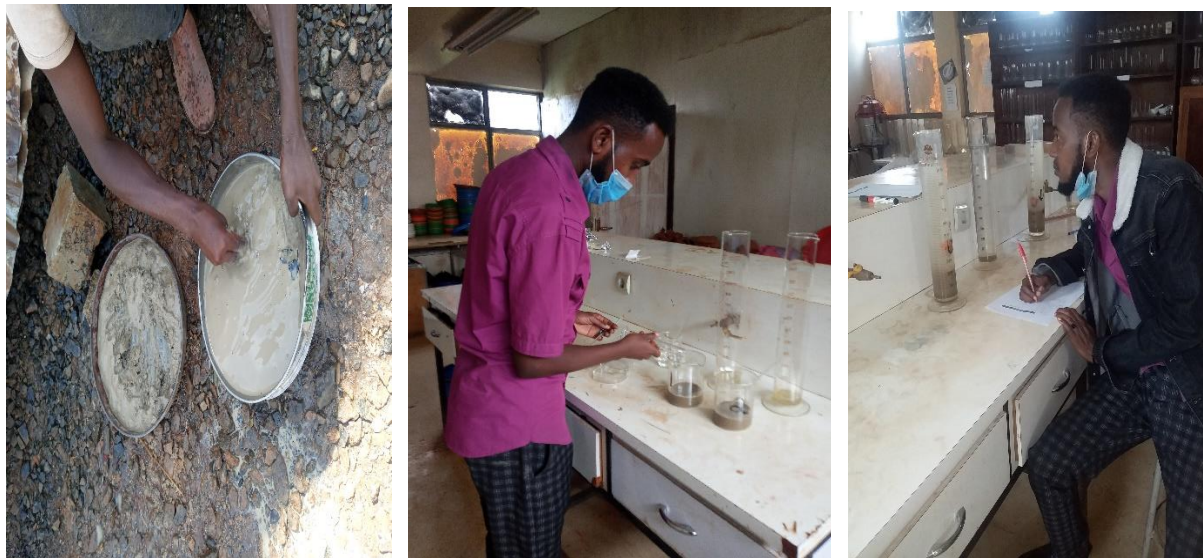
Figure 3.6 Photo of both wet sieving and hydrometer analysis (Picture taken by Ahmed)
