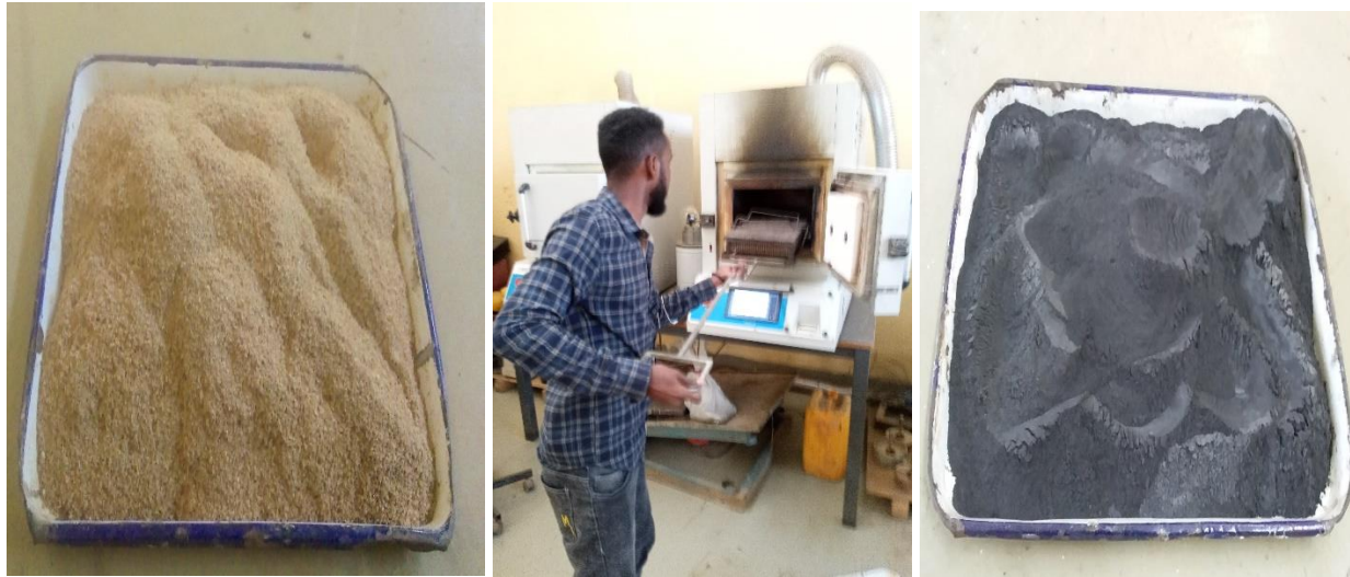
Figure 3.3 Process of Sorghum Husk Ash (SHA) preparation (Picture taken by Eyuel)
