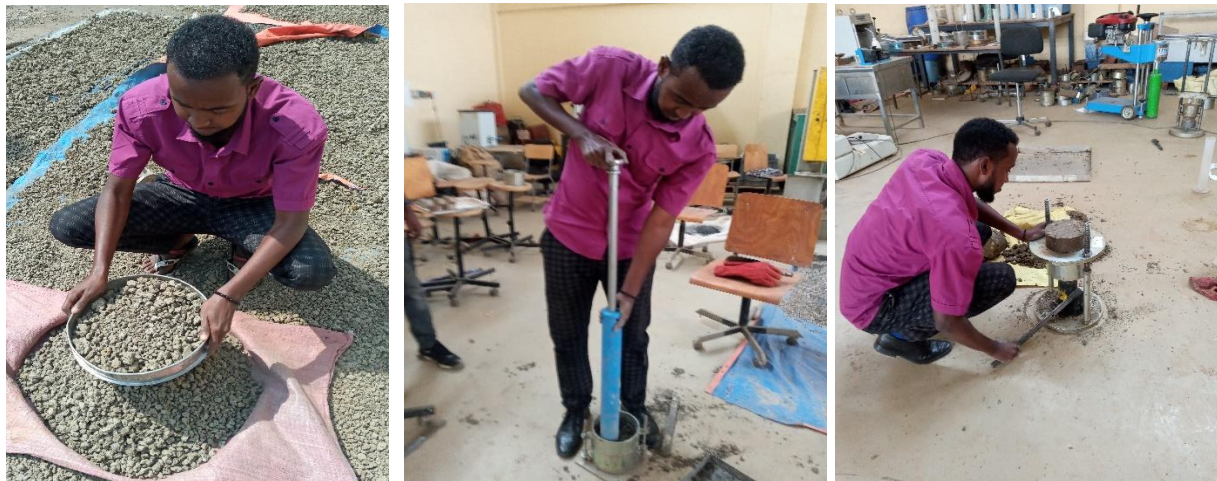
Figure 3. 11 Photo Compaction test and procedures (Picture taken by Ahmed)
