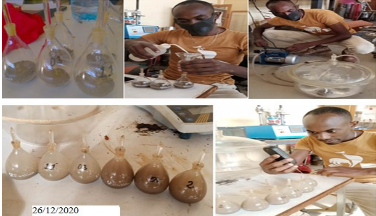
Figure 3.9: Specific gravity test
