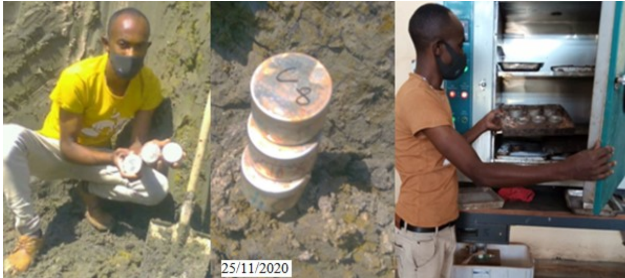
Figure 3.4: Sampling and test for natural moisture content
