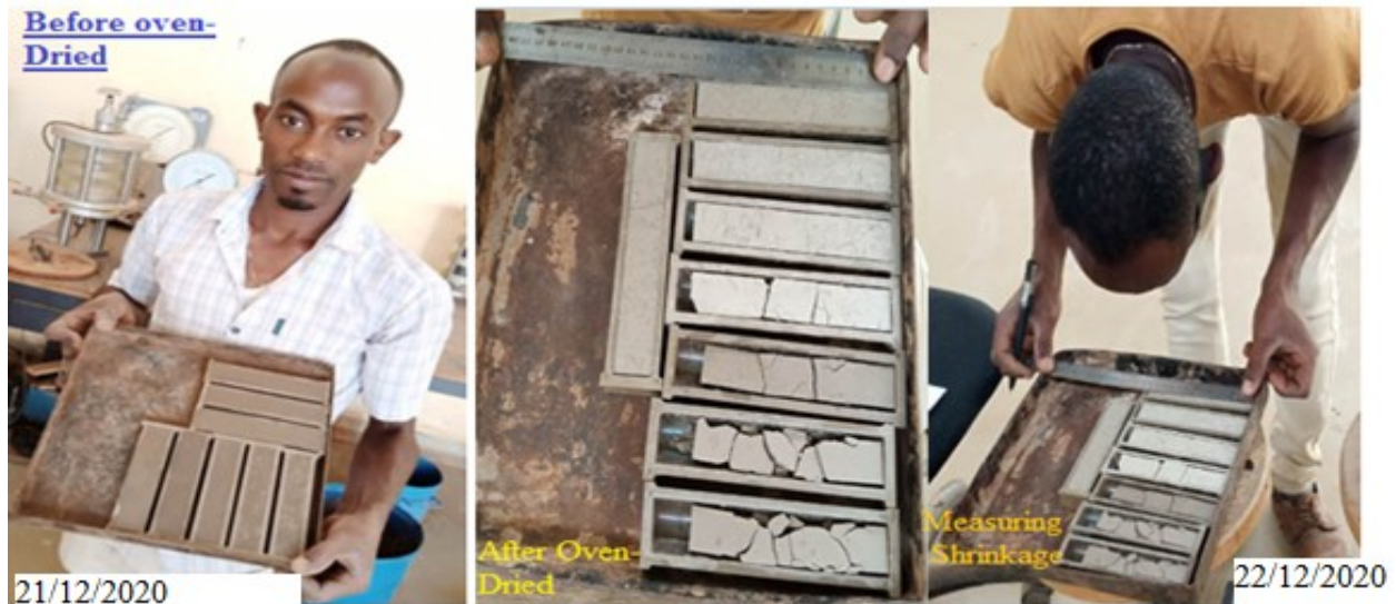
Figure 3.8: Linear shrinkage test
