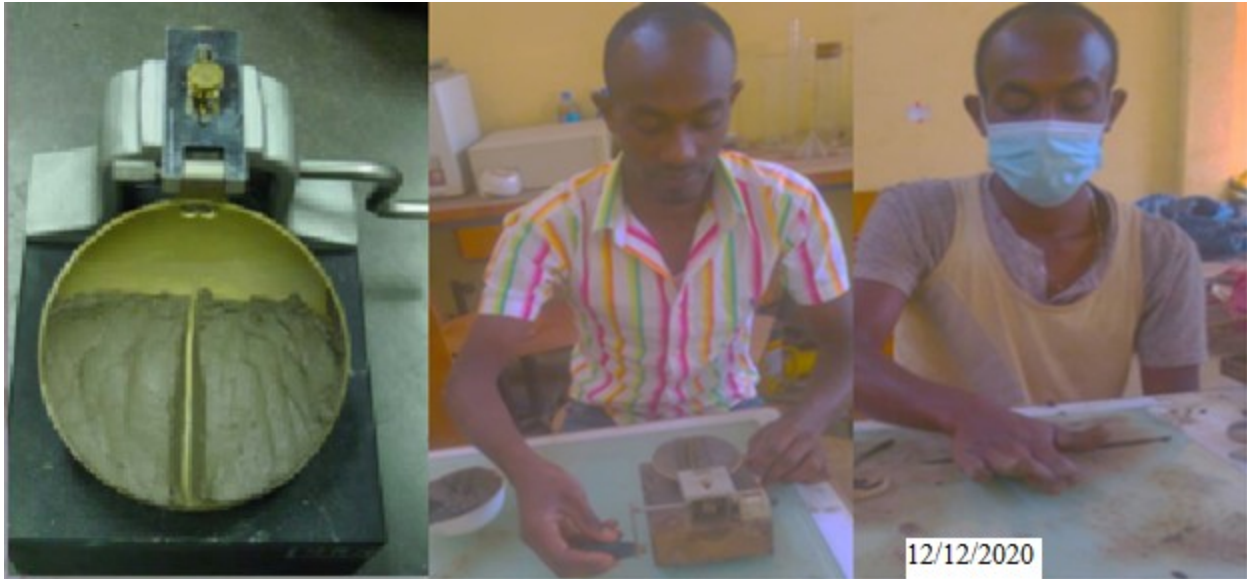
Figure 3.5: Atterberg limits test
