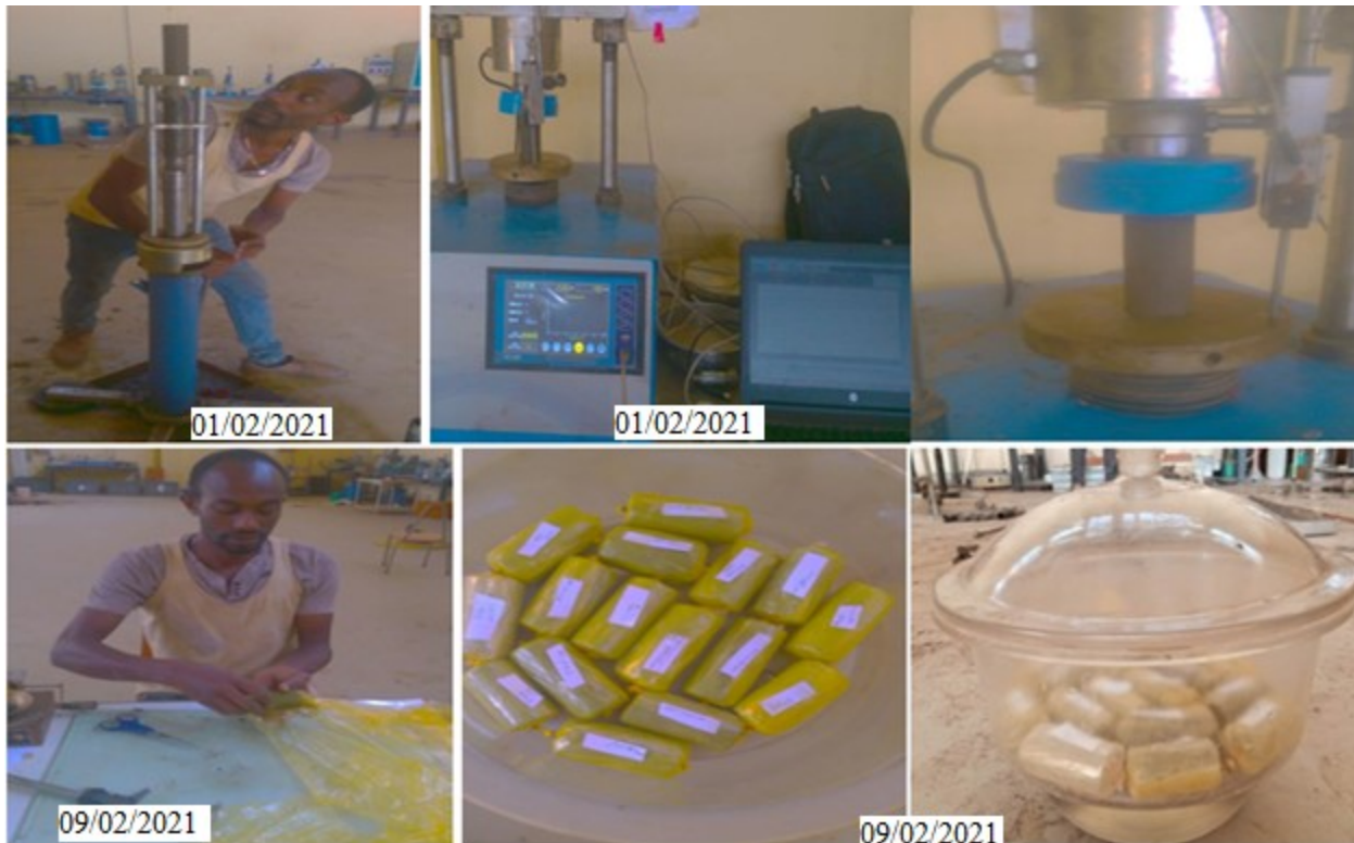
Figure 3.12: UCS (Unconfined compression strength) test
