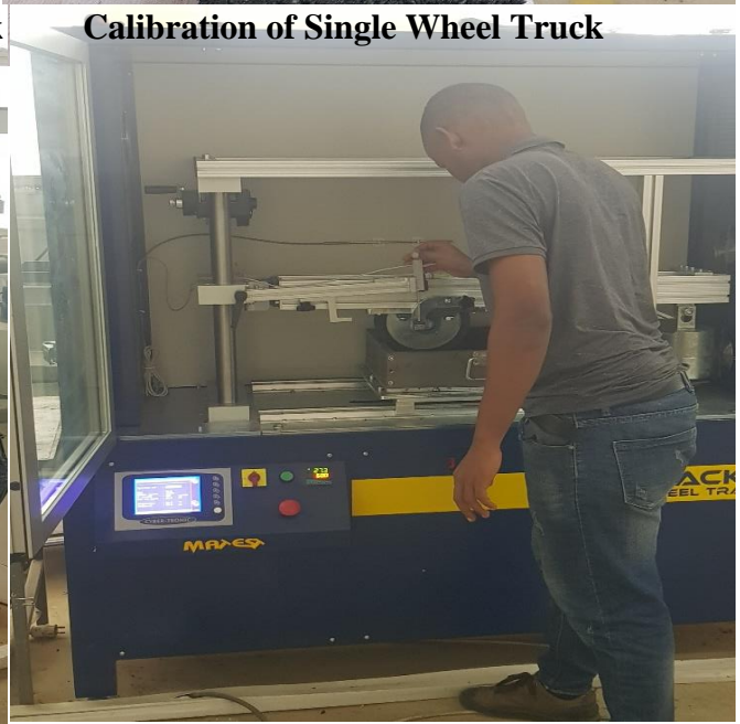
Rutting Depth Test by Single Wheel Truck
