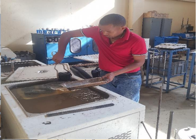
Compacted Specimen in Water bath
