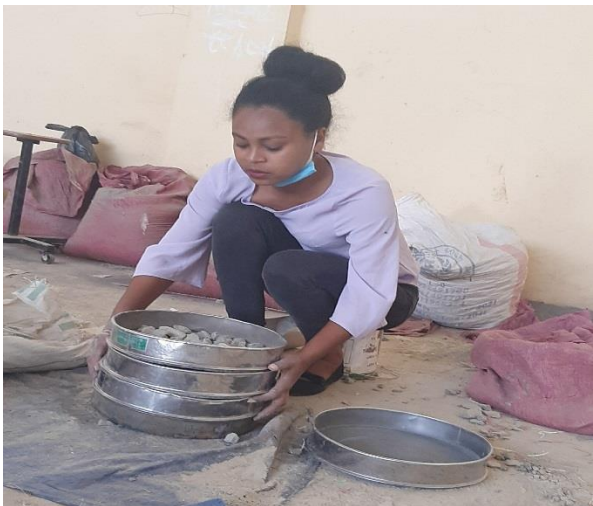
Sieve the aggregates to get crushed stone dust filler
