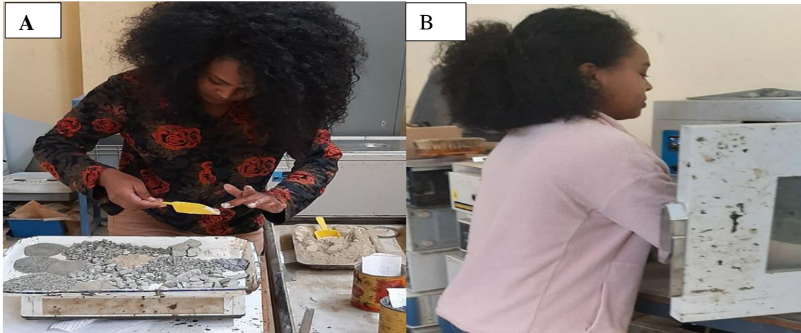
Figure 3.6: Preparation of sample for Marshall Mix design (picture taken on 9/05/2021)
