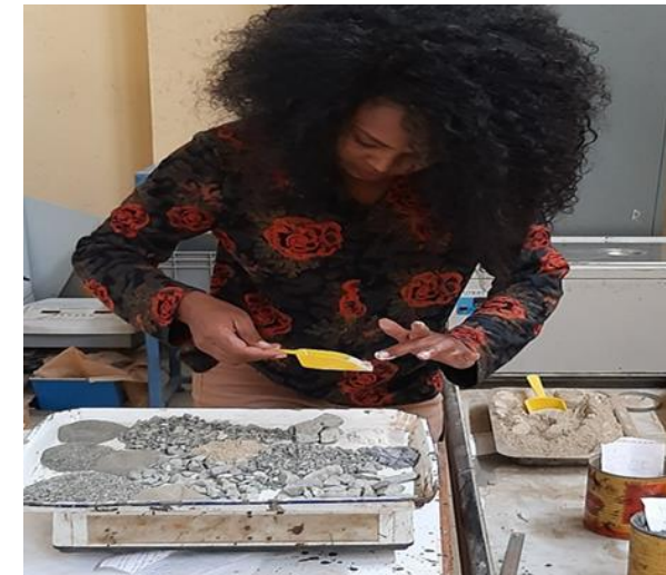
Prepare the aggregates for Marshall Mix
