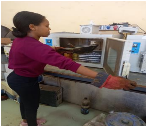
Put the aggregate and fillers in oven and then mix
