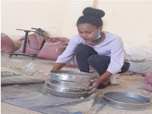
Sieve the aggregates to get crushed stone dust filler
