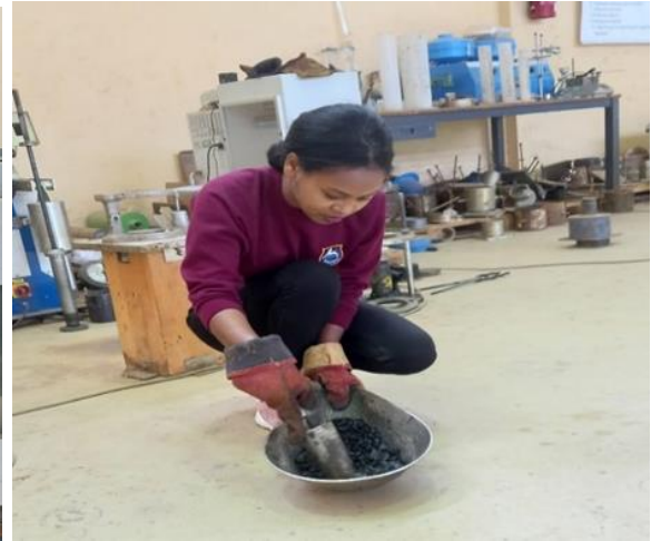
Put the aggregate and fillers in oven and then mix
