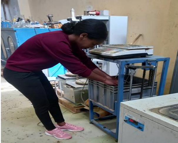
Weighting the specimen in water and after drying by cloth
