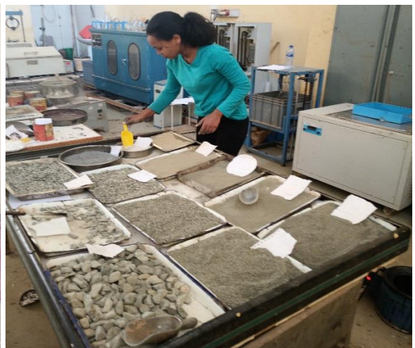
Sieve the aggregates to get crushed stone dust filler
