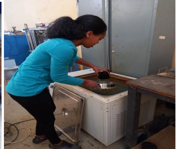
Put the specimen in water bath and ready for flow and stability test results
