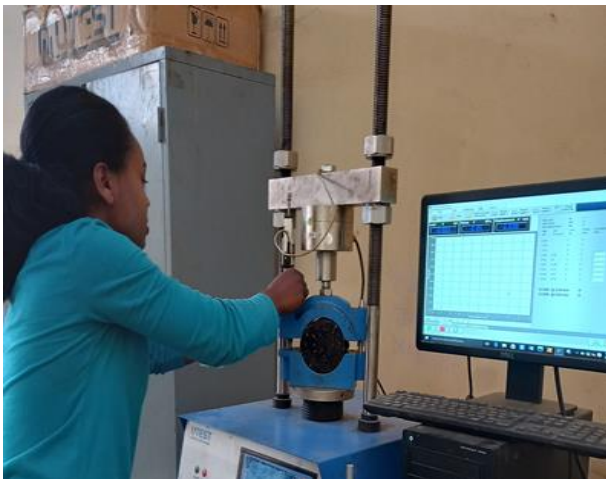
Recording the flow and stability test results
