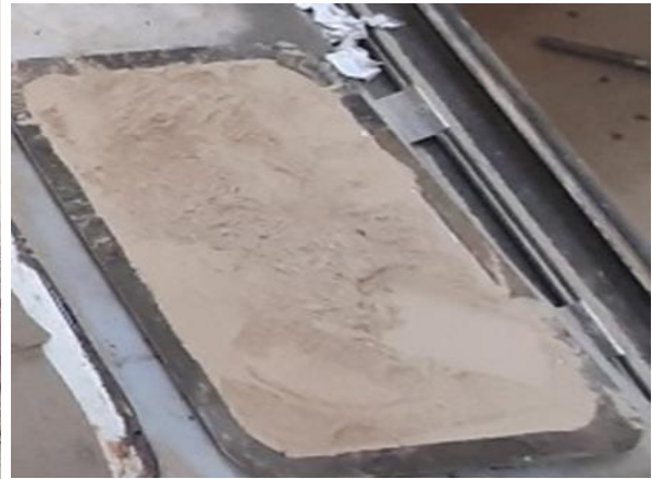
Sieve the aggregates to get crushed stone dust filler
