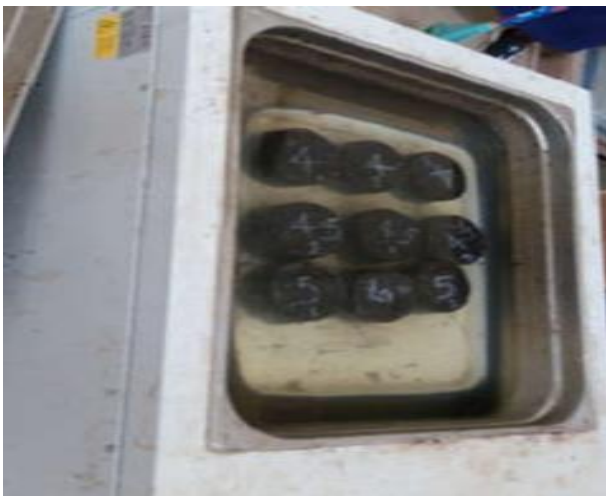
Put the specimen in water bath and ready for flow and stability test results
