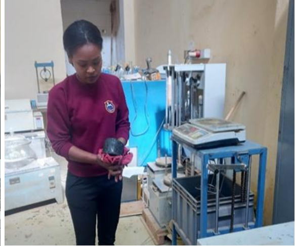
Weighting the specimen in water and after drying by cloth
