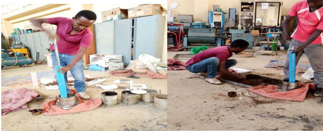
Figure 3.6 Modified compaction and CBR compaction (Haile Zenebe July 1/2021)
