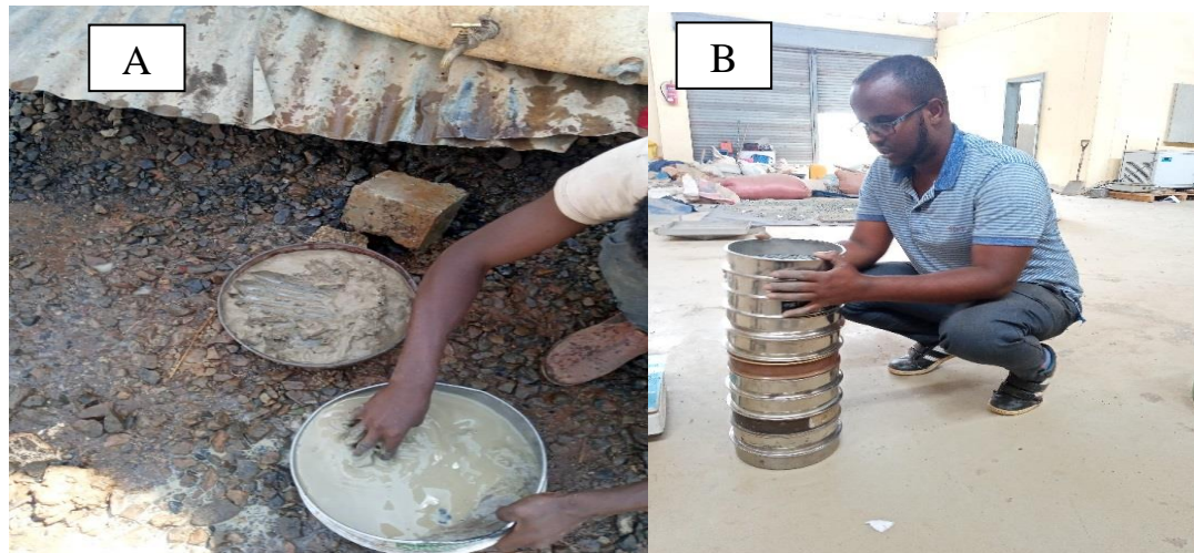
Figure 3.6: Wet sieve analysis Test (A) washing the soil (B) Sieving the dry soil (Captured by Abdirahman.A, 19/03/2021)
