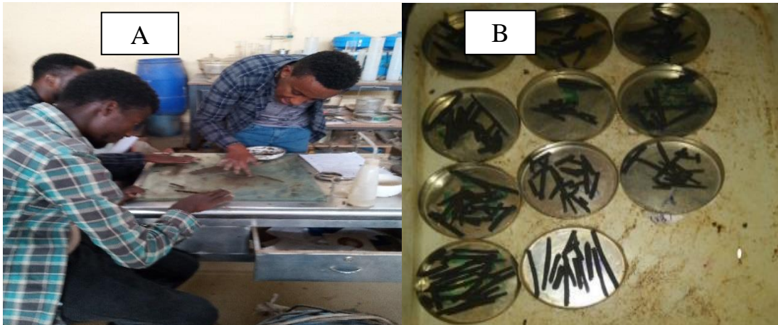
Figure3.10: Plastic limit Test (A) paste sample is rolling and (B) Crumbling soil (Captured by Ahmed.M, 22/02/2021)
