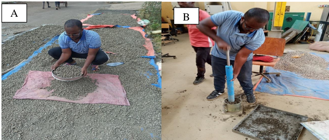
Figure 3.13: Compaction Test (A) Sieving the sample and (B) Compacting the sample (Captured by Abdirahman.A, 30/02/2021)
