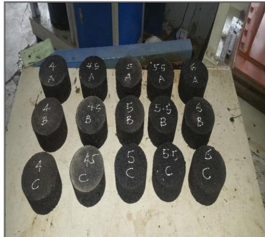
Sample prepared to stability test
