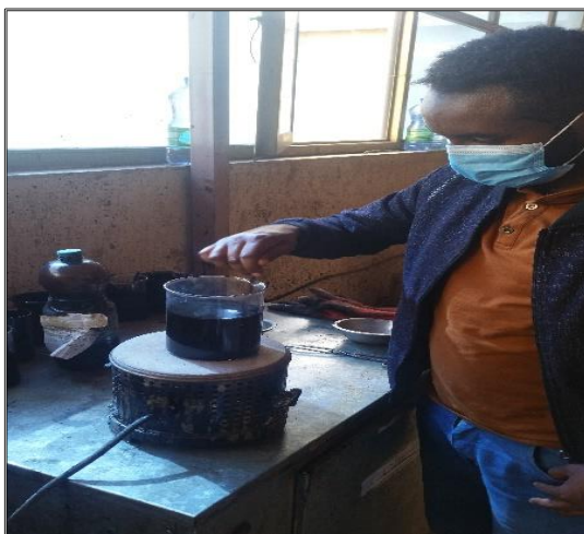
Prepare Modified Bitumen with Crumb Rubber
