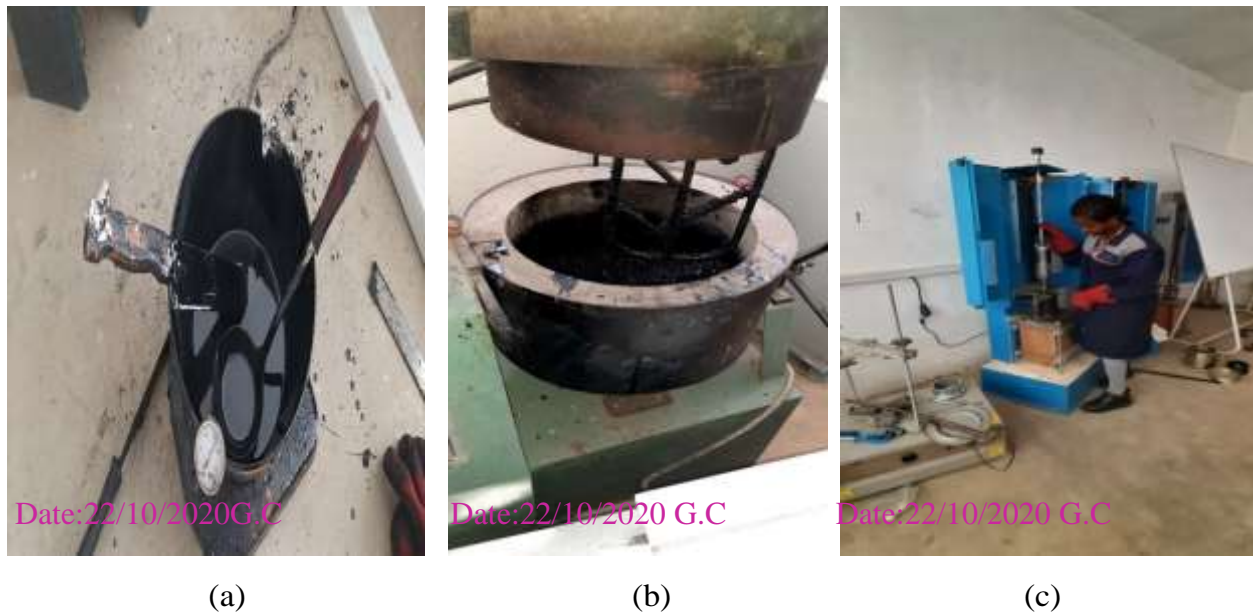
Figure 3.13: Heating of Bitumen, (b) Mixing of HMA Specimen, (c) HMA Compaction
