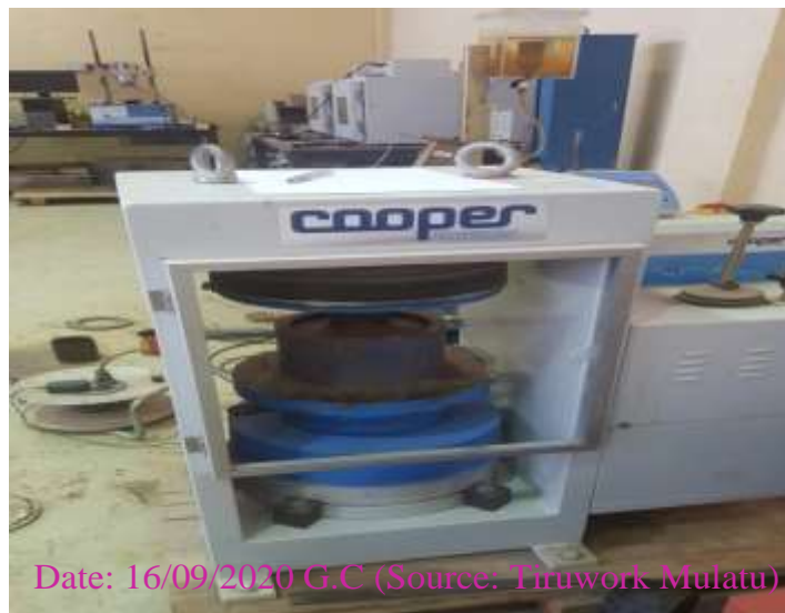
Figure 3.6: Aggregate Crushing Value Test
