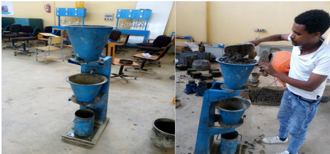
A) Compaction factor test apparatus B) fresh concrete added to the compaction test apparatus
