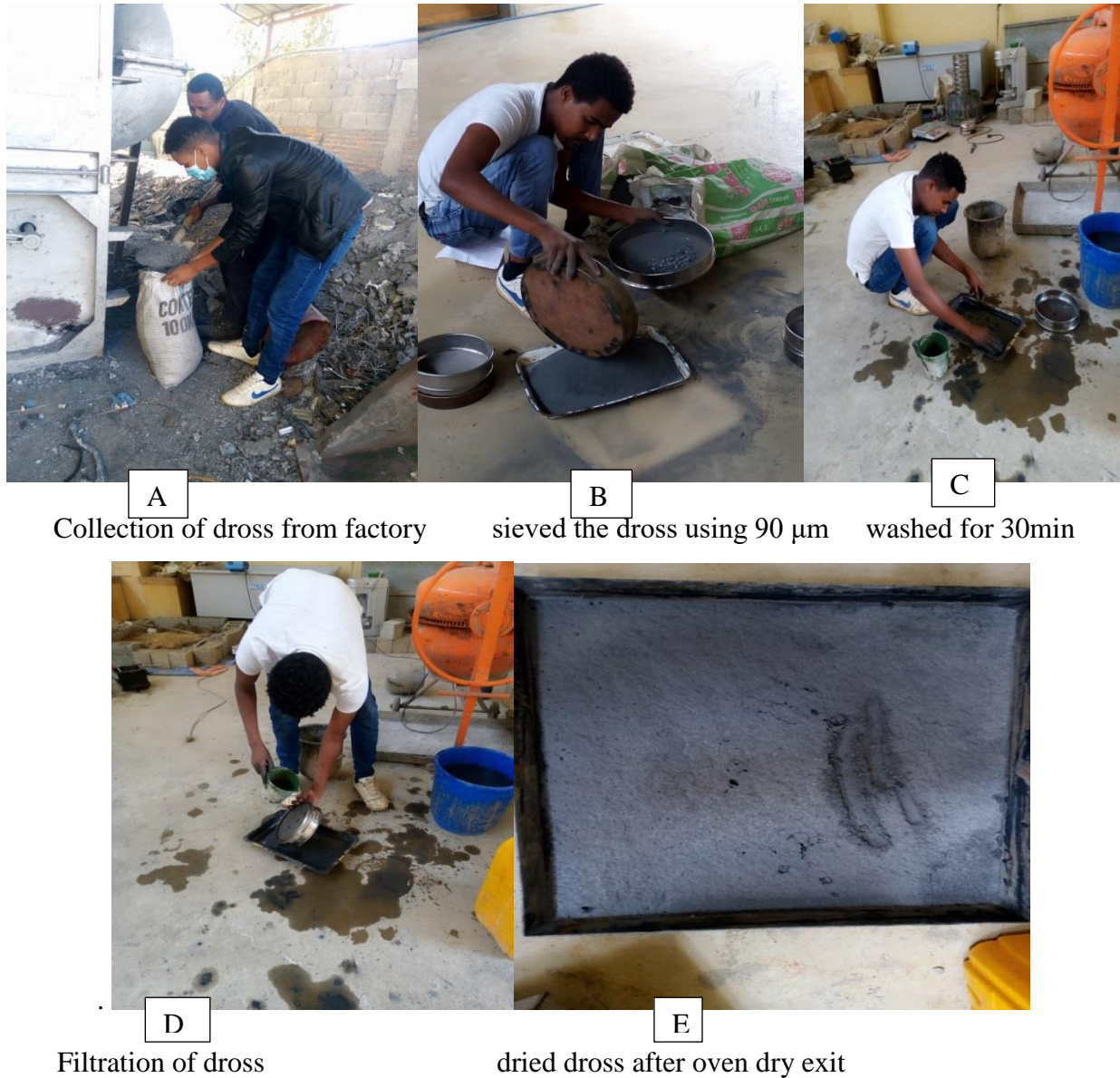
Figure 3.5 Photos shows the steps of SAD preparation
