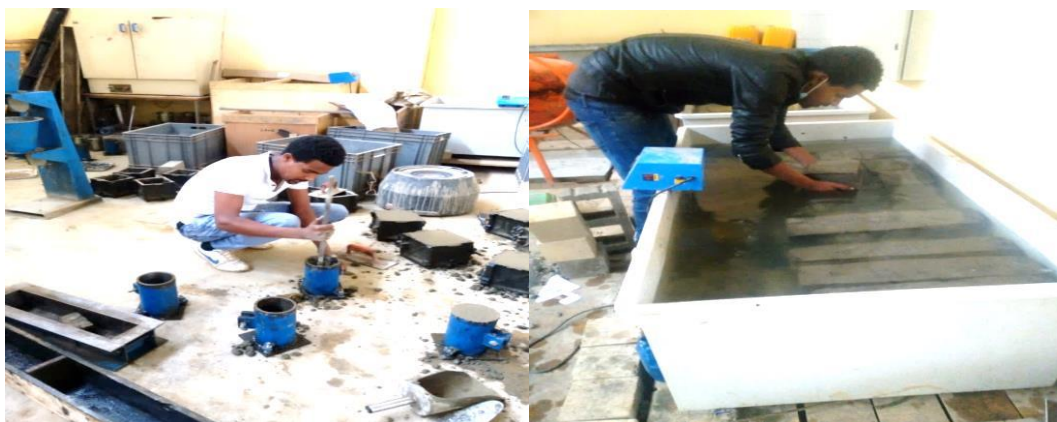
A) Compacting using metal rods
