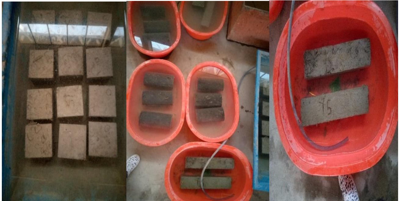
Figure 6. Cube, Cylindrical and Prism Sample in Curing Bath.
