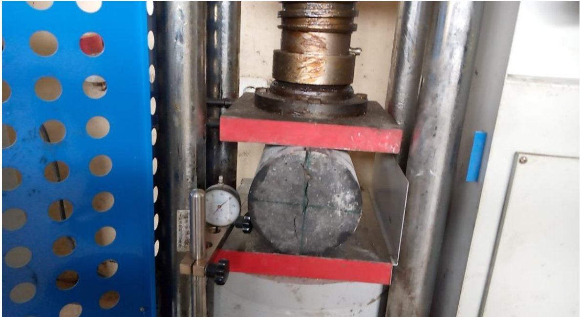
Figure 9. Concrete cylinder setup for split tensile test
