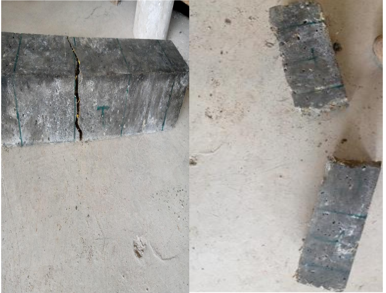
Photo: Line of beam failure under third-point loading flexural strength testing
