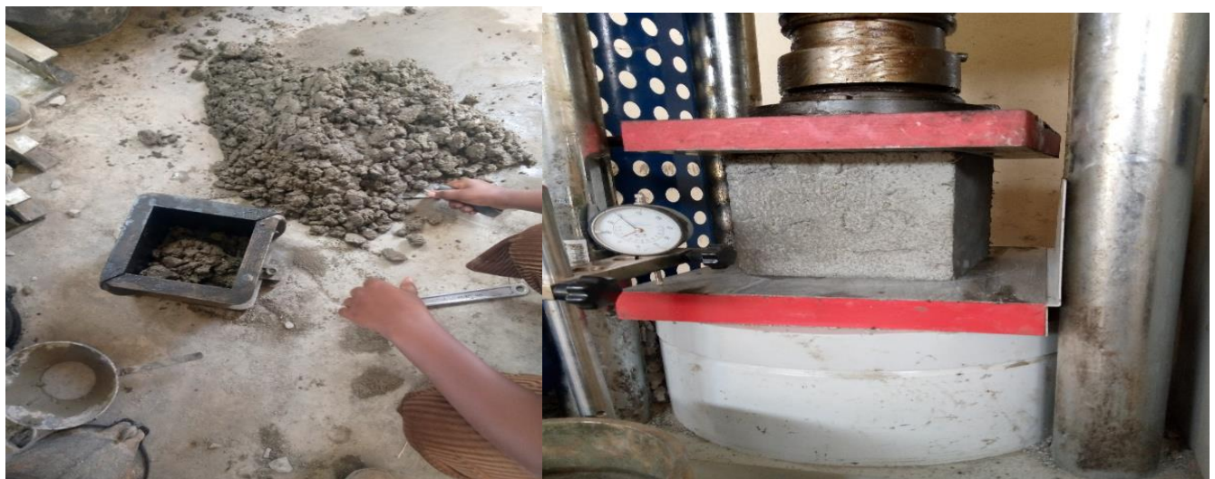
Figure 7. Casting and Testing for Compression Test.
