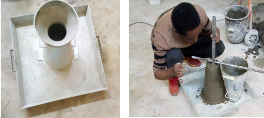
Figure 3.4: Slump test on concrete
