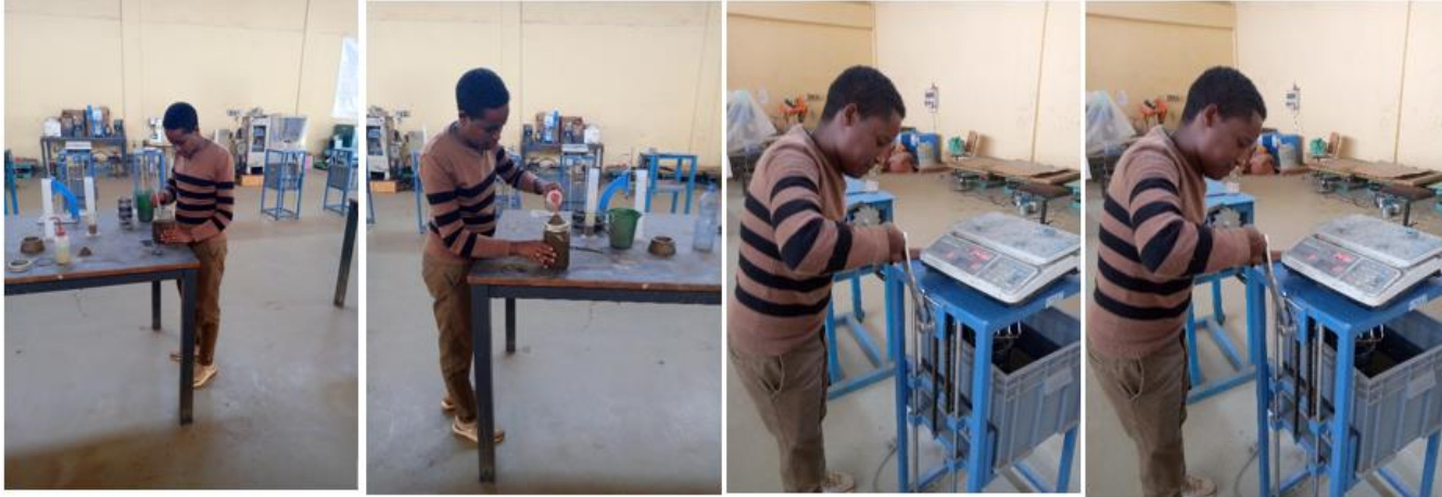
Photo-6 Specific gravity test for fine and coarse aggregate
