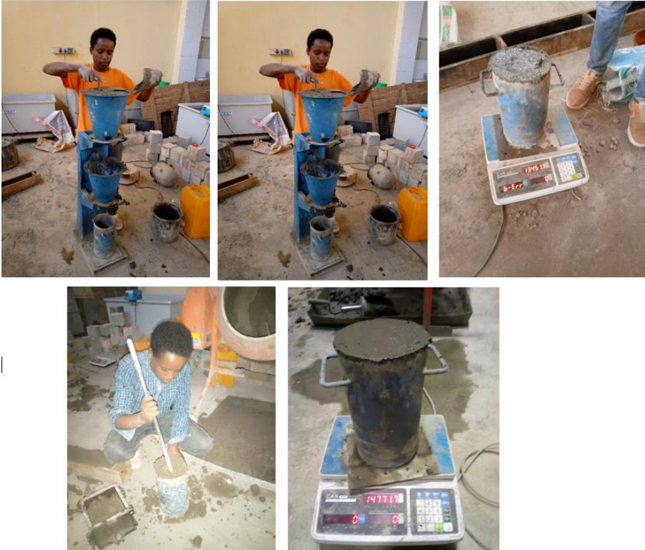
Photo-11 Fresh Concrete Properties Compaction Factor Test
