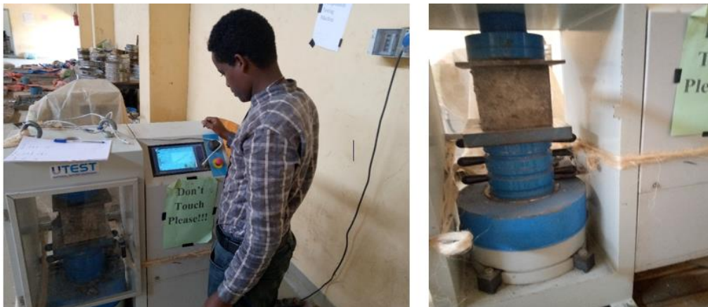
Figure 3.8: Cube tested on compression testing machine.
