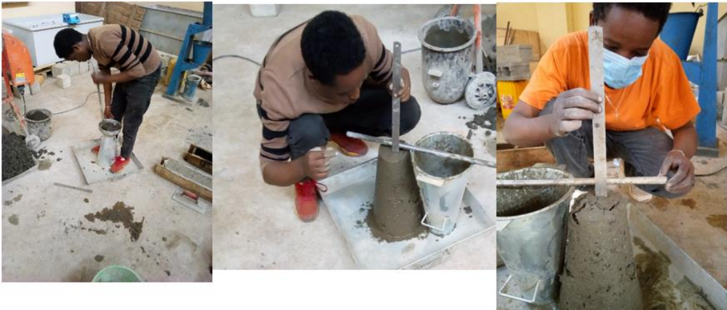
Photo-10 fresh concrete properties slump test
