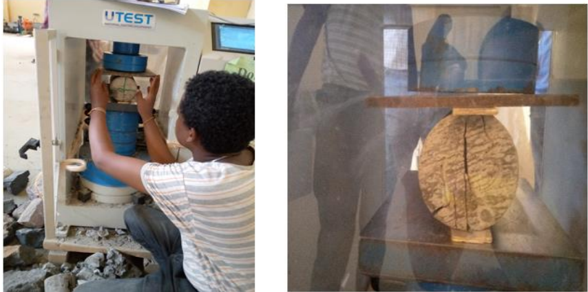
Figure 3.9: Split tensile strength test setup
