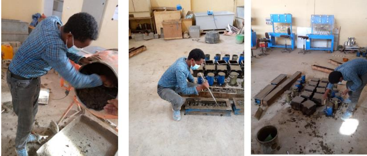
Figure 3.6: Mix and casting
