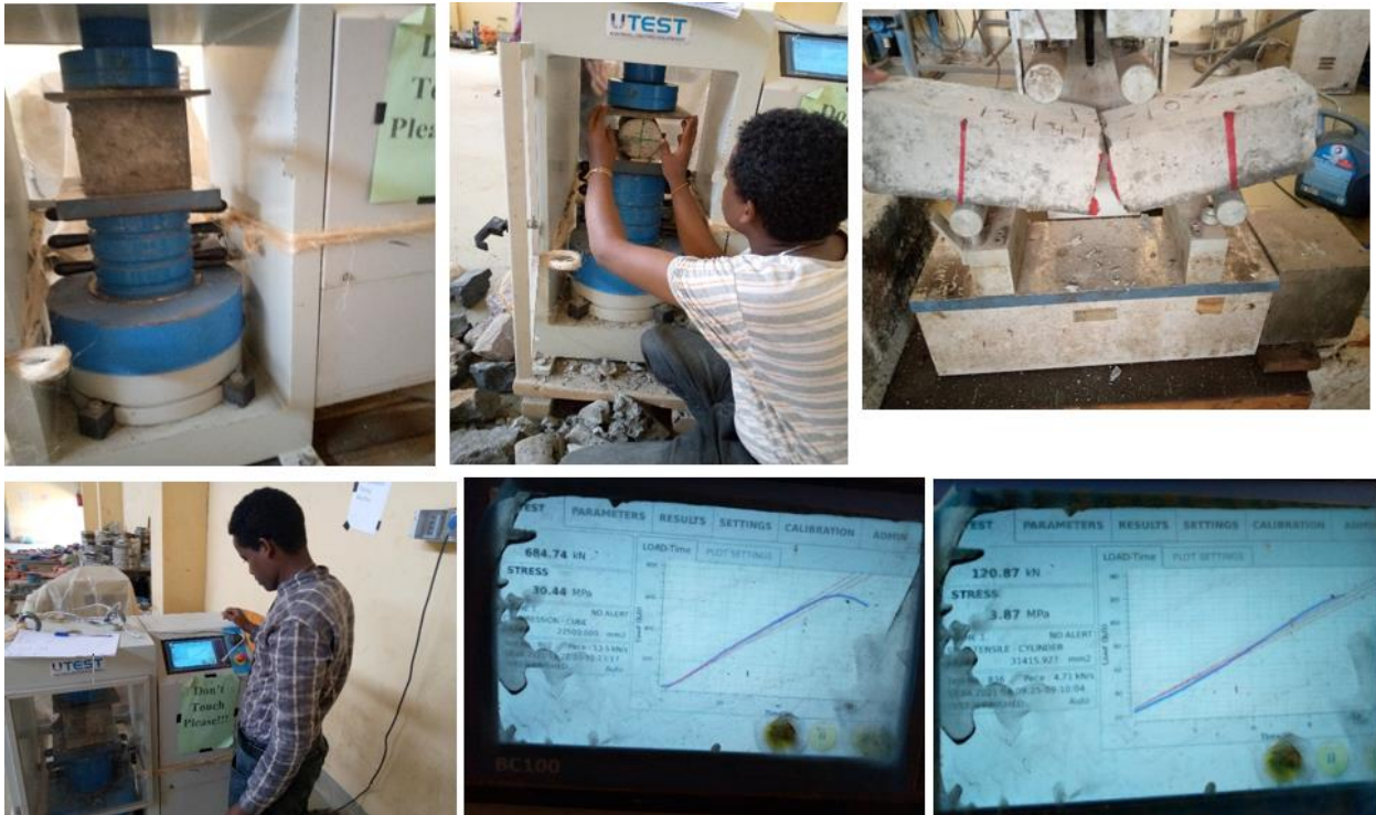
Photo-14 During hardened concrete test
