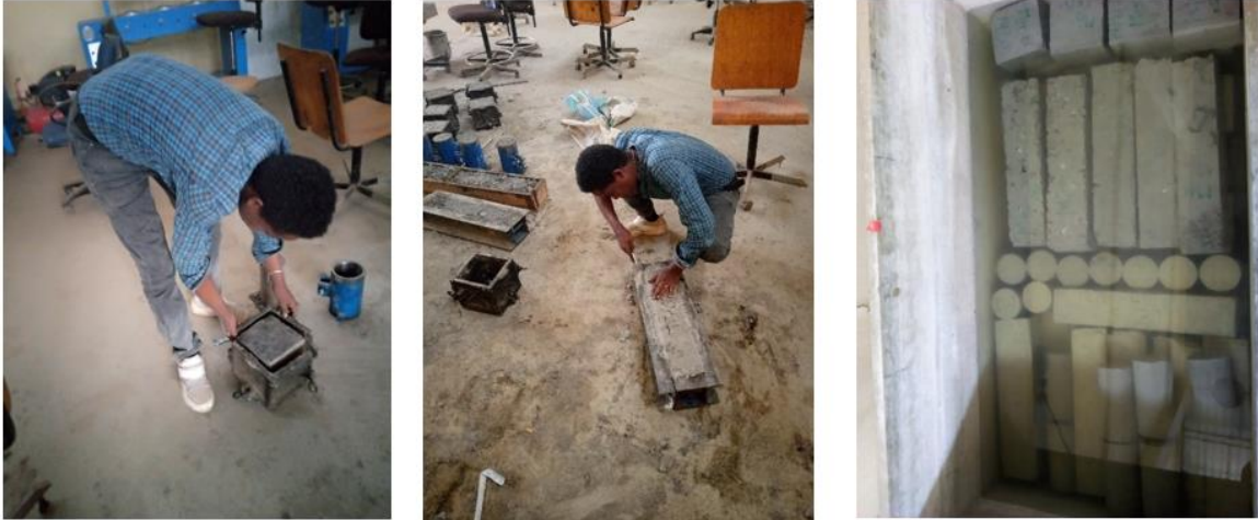
Figure 3.7: Demolding and curing Casted specimen
