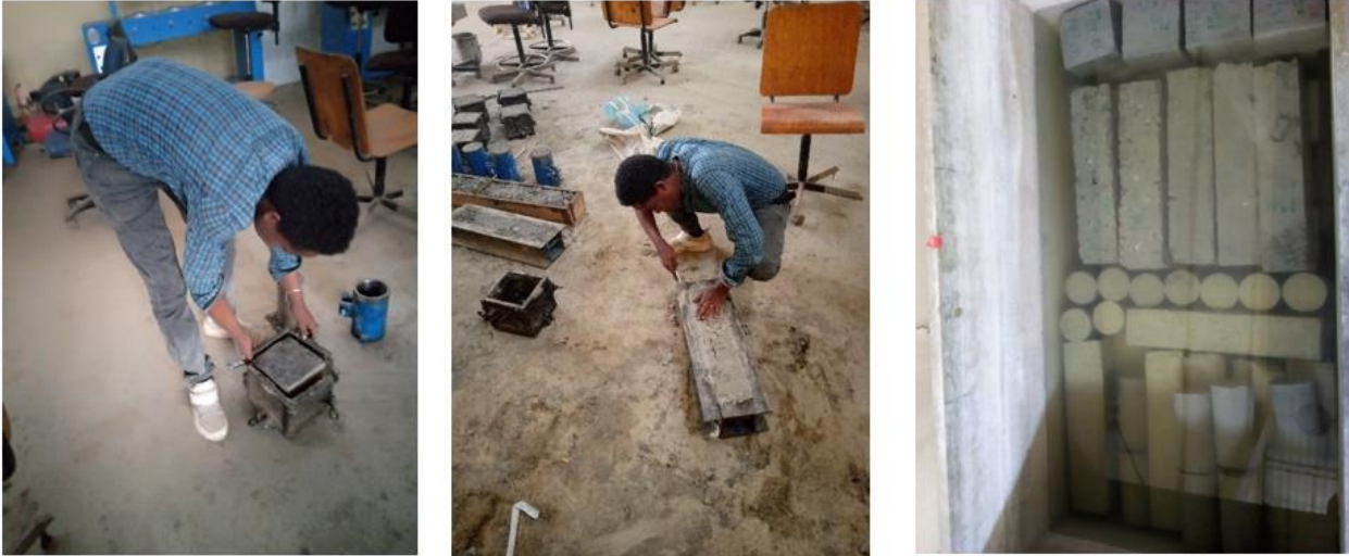
Photo-12 Demolding and curing Casted specimen
