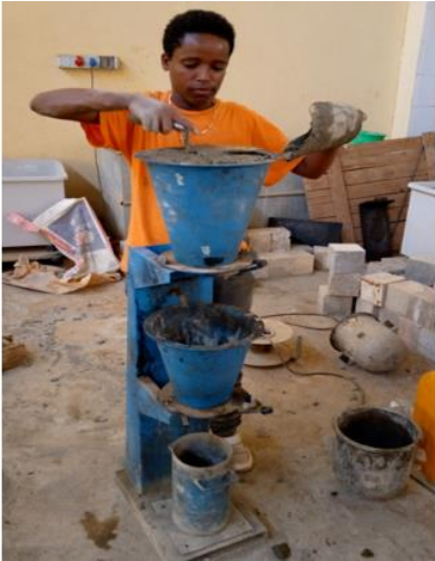
Figure 3.5: Compaction Factor test on concrete
