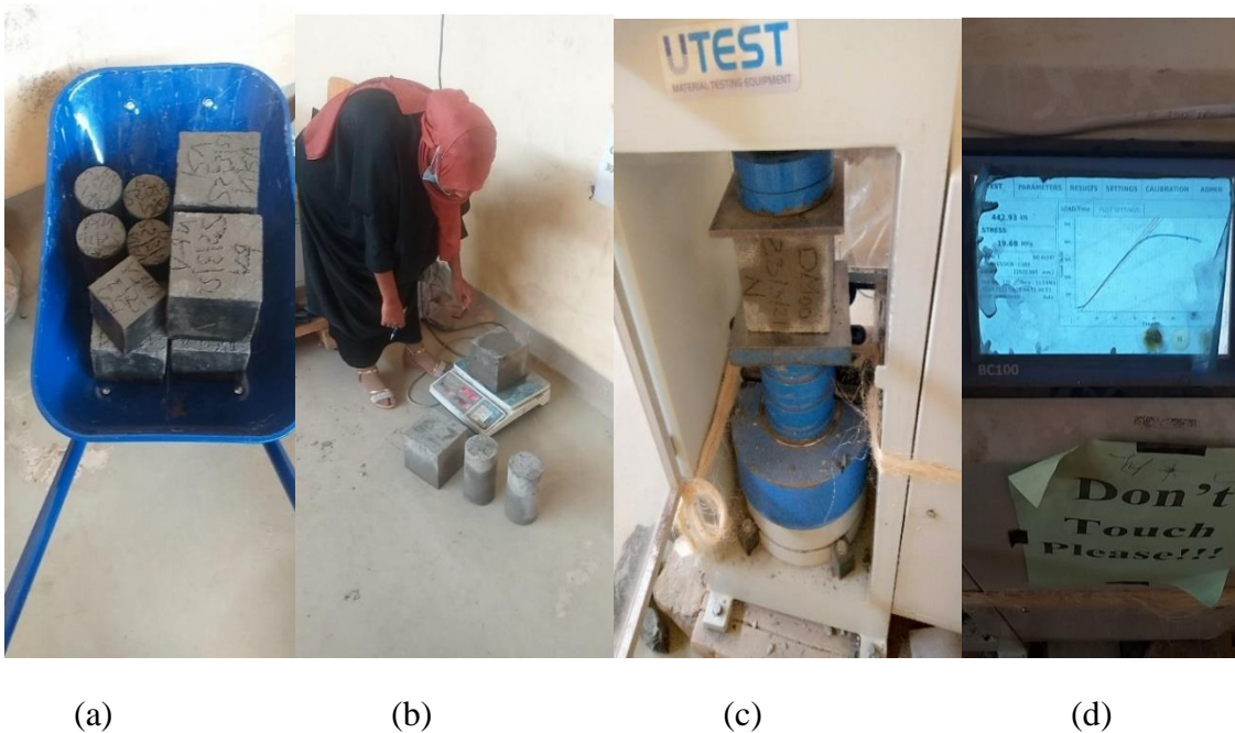
Figure 3.12: (a)After curing (b) Weighting the cube (c) Cube test and (d) Result display
