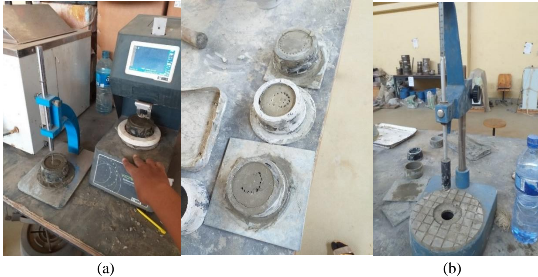
Figure 3.11: (a) Setting times tested both manually and automatic and (b) Penetration depth measurement
