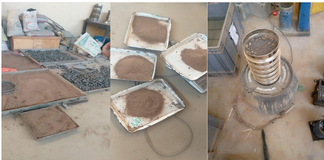
Figure 3.5: (a) Air drying sand (b) 2kg weigh sand and (c) Sieve analysis of sand.
