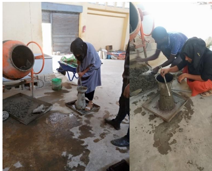
Figure 3.10: (a) Compact and (b) Measuring the slump height
