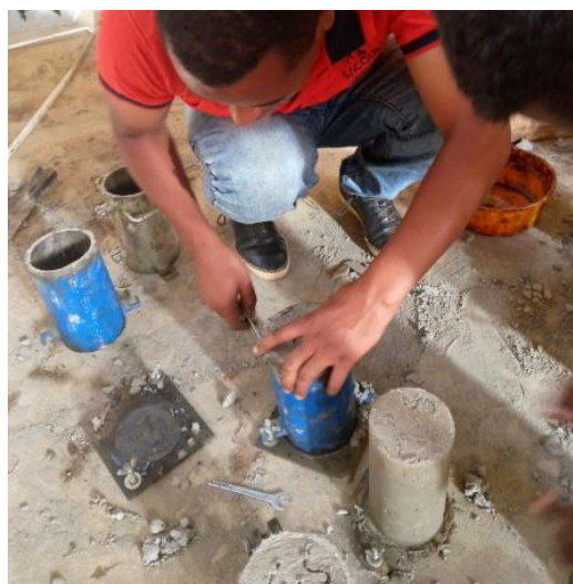
Figure 3-23: Demolding specimen for curing
