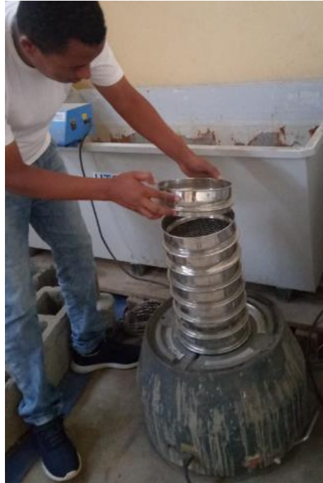
Figure 3-9: Arranging of sieves for sieve Analysis of Fine Aggregate
