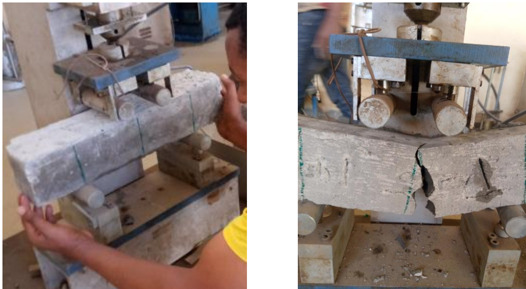
Figure 3-21: Flexural strength setup and crack pattern due to loading
