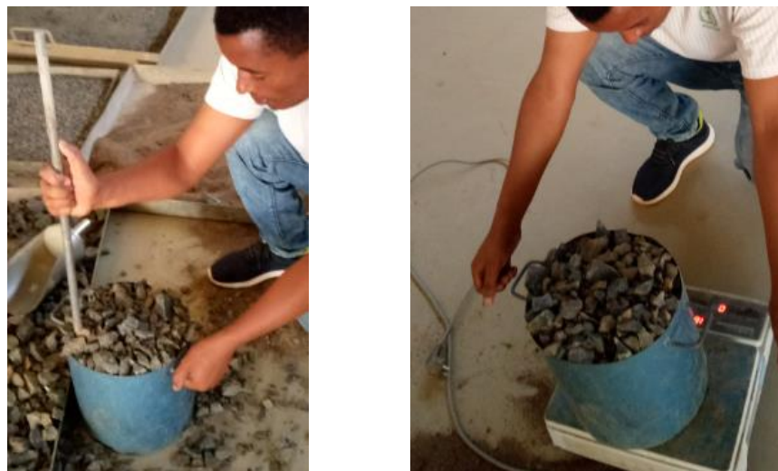
Figure 3-14: Compacting and balancing the mass of Compacted Coarse Aggregate
