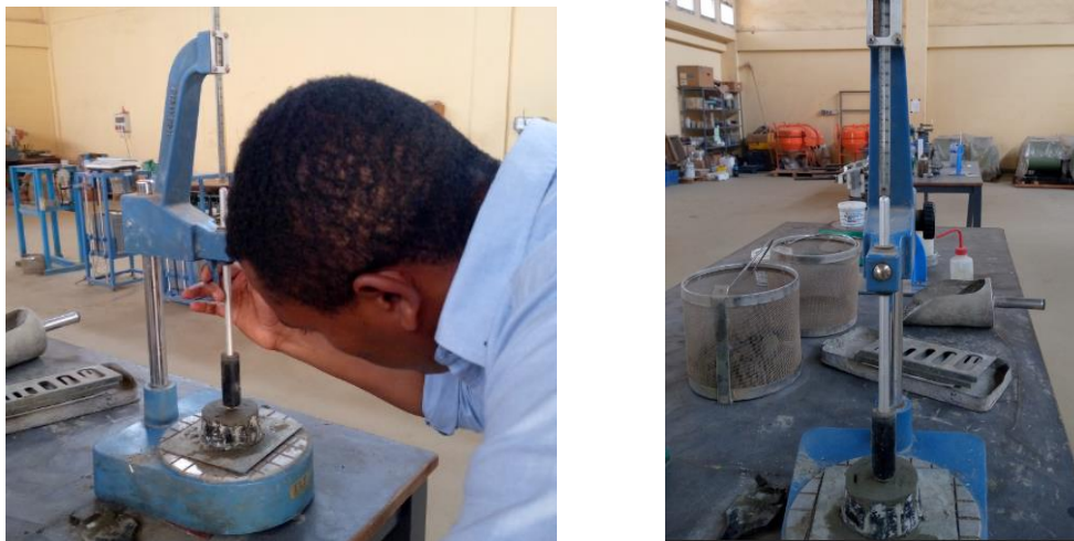
Figure 3-5: Asymptote the plunger to paste and measure penetration depth after 30second
