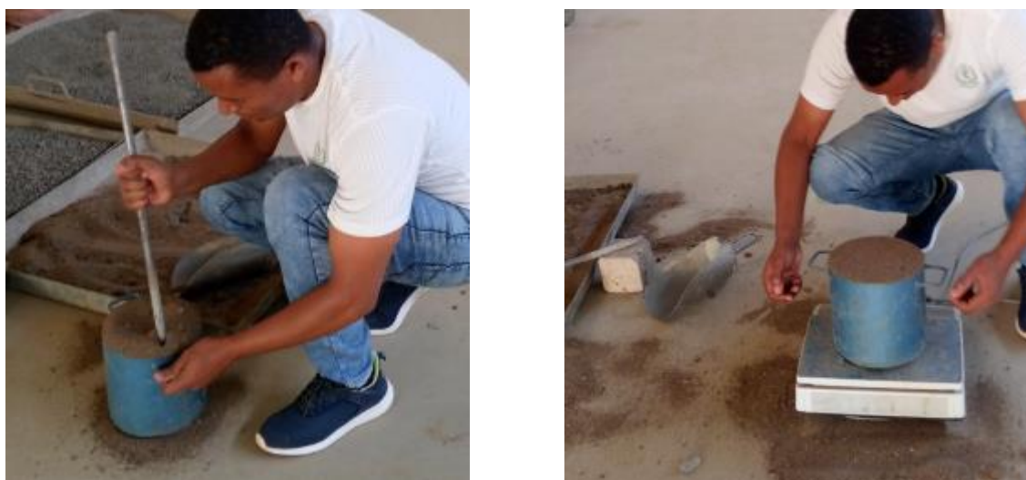
Figure 3-11: Compacting and balancing the mass of Compacted Fine Aggregate
