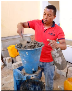
1 st add fresh concrete to cones
