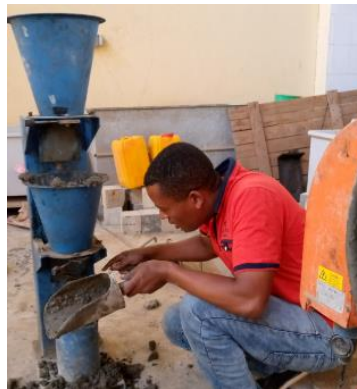
2 nd pass concrete to cylinder
