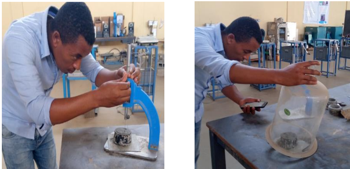
Figure 3-7: Measuring penetration depth after putting under cabinet for 30minutes
