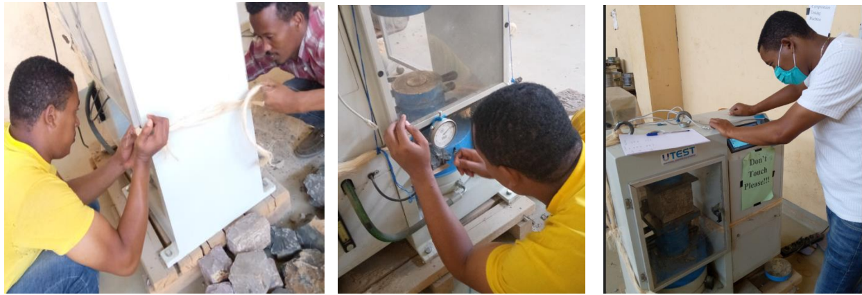
Figure 3-18: setting dial gauge and Record load for interval of each 50 count of the dial
