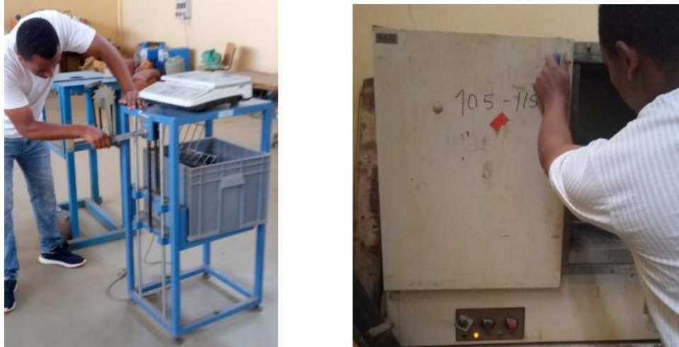
Figure 3-13: Jolting of saturated Coarse and inserting to oven of surface dried Coarse Aggregate
