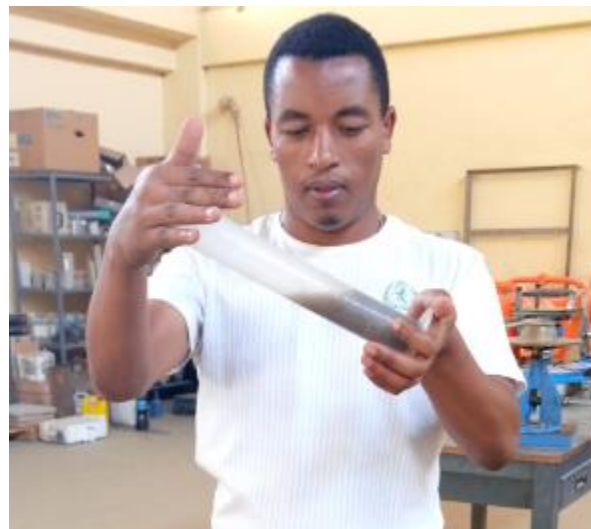
Figure 3-8: shaking sample of fine aggregate in jar to determine silt content
