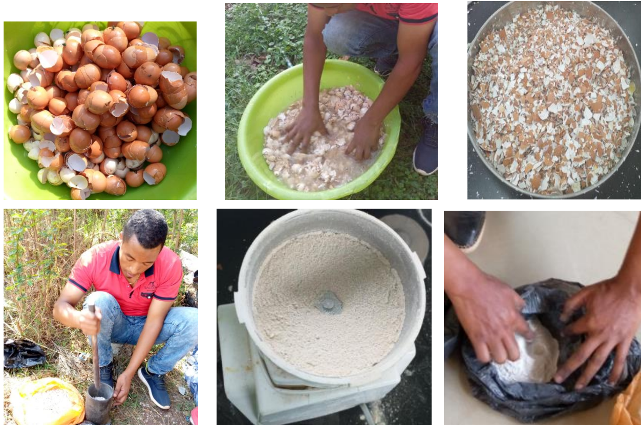
Figure 3-3: Procedural Preparation of eggshell powder
