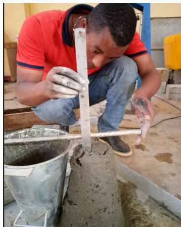
Figure 3-15: Measuring Slump of fresh concrete
