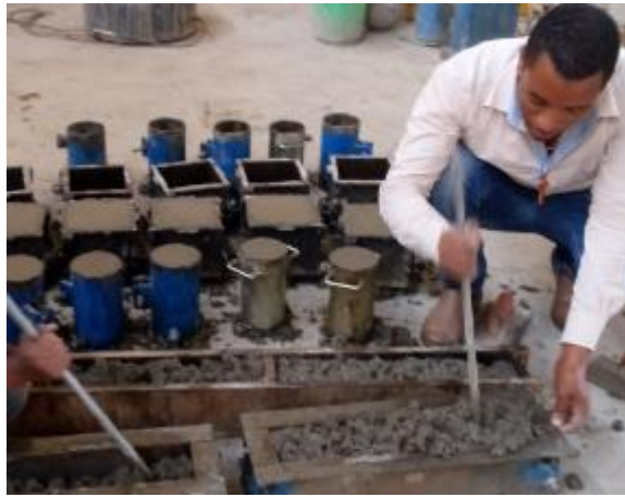
C. Compacting of fresh concrete
