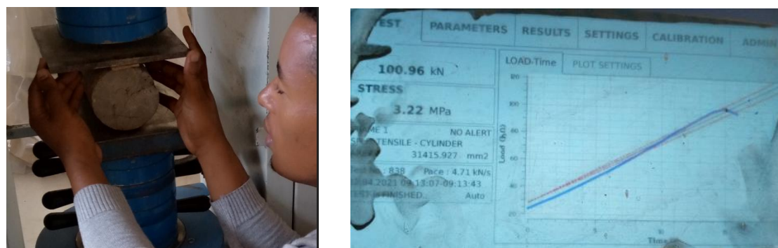
Figure 3-20: Splitting tensile strength test setup and sample test result
