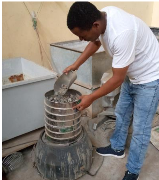
Figure 3-12: Adding of sample of Coarse Aggregate for sieve Analysis
