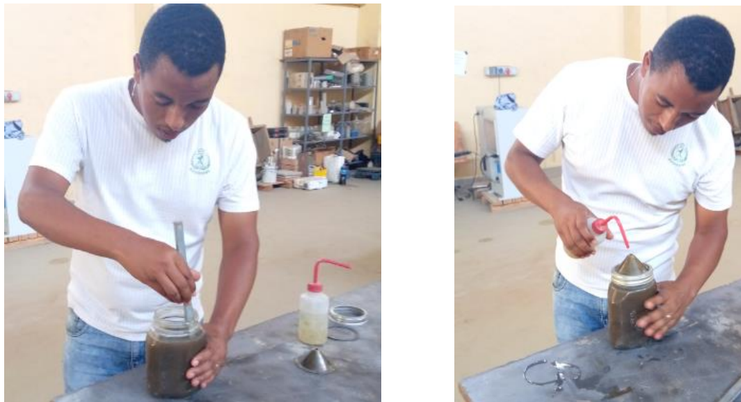
Figure 3-10: Removal of air bubbles by using rod and fill with water the pycnometer
