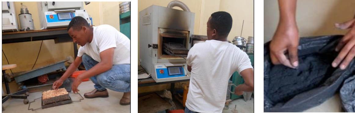
Figure 3-4: Procedural Preparation of Sawdust ash
