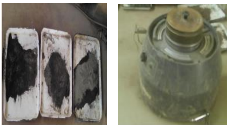
Figure 3-6: Samples for testing Fineness of samples and sieving for 15minutes
