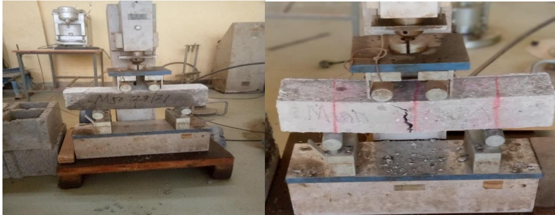
Figure 3: 9 Center point loading flexural strength test
