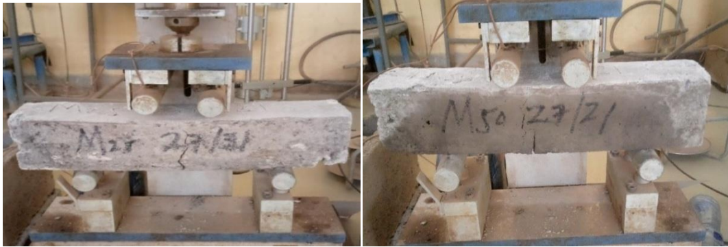
Figure 4- 15: Crack and failures observed CW and SD beam
