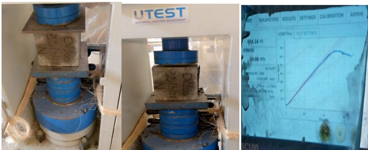
a) Cube specimen ready for test b) concrete cube sample after test (c) stress from UTM
