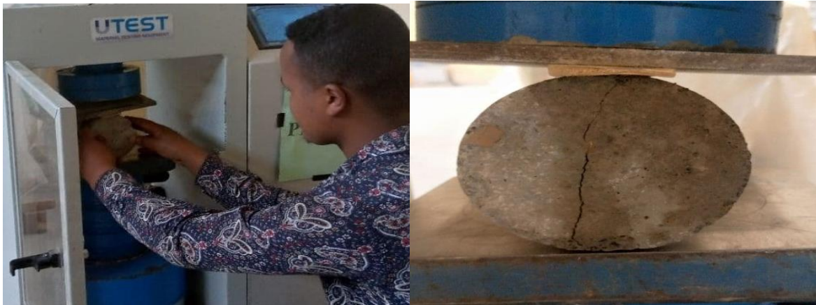
Figure 3: 10 Splitting tensile strength of specimen
