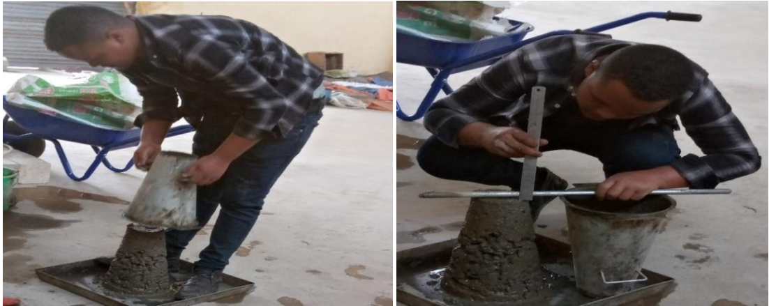
Figure 3: 6 Slump test of concrete
