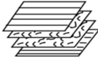
Figure 2. 1 Figure laminar composite redrawn from [32]
