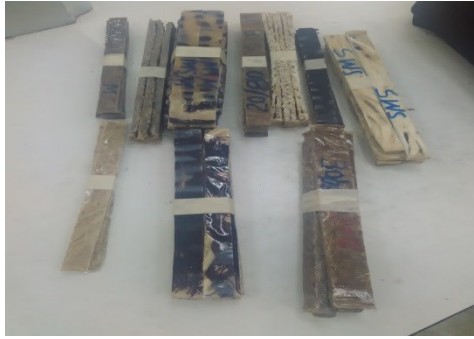
Figure 3. 12 Specimen prepared for tensile test
