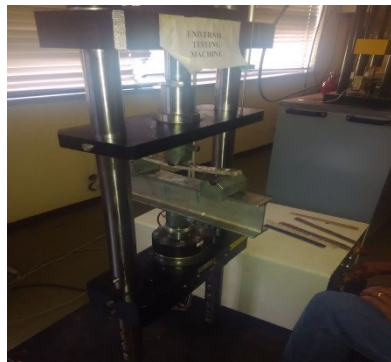
Figure 3. 15 Flexural test set up
