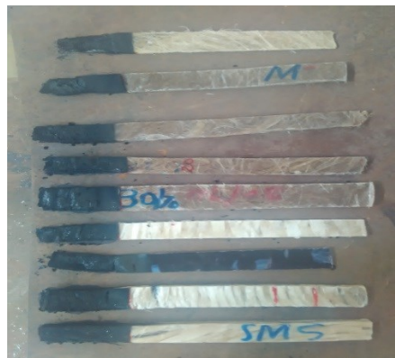
Figure 4. 1 Remains of the samples after the burning test.
