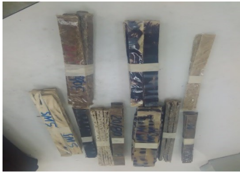
Figure 3. 13 Specimen prepared for flexural test
