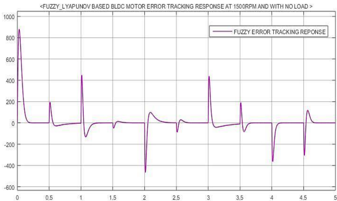
Figure 49: No load error tracking response of Fuzzy based MRAC system at 1500rpm rated speed.
