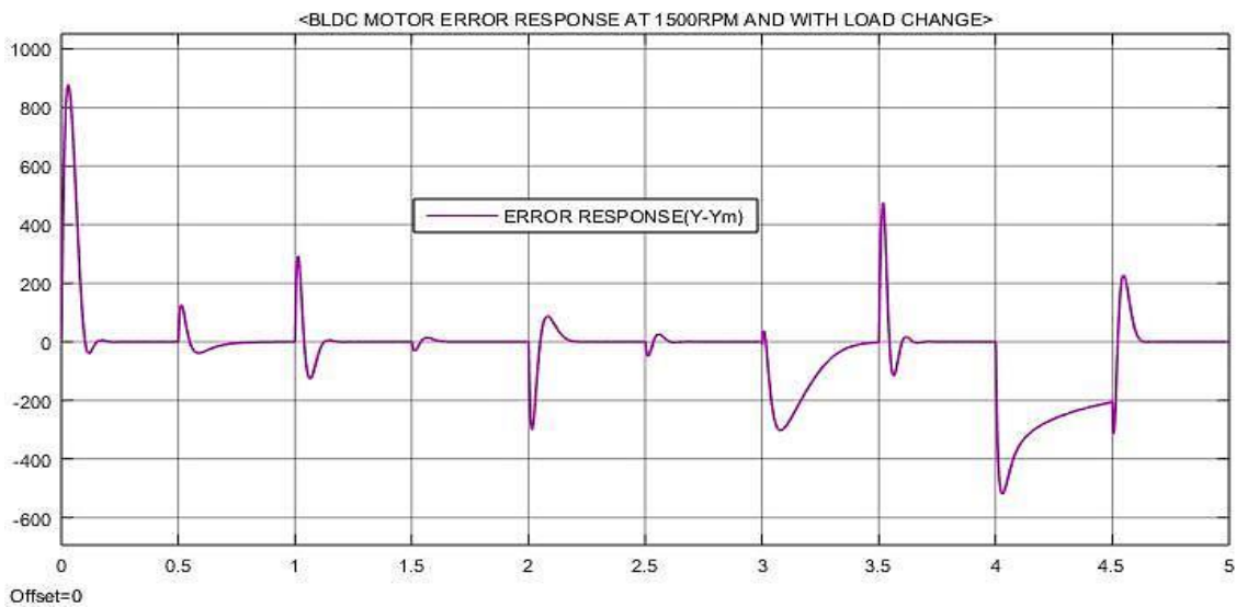
Figure 38: Lyapunov stability method sudden load change, tracking change in error response at 1500rpm.
