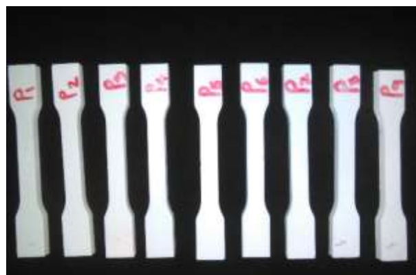
Figure 2: Parts fabricated by FDM machine
