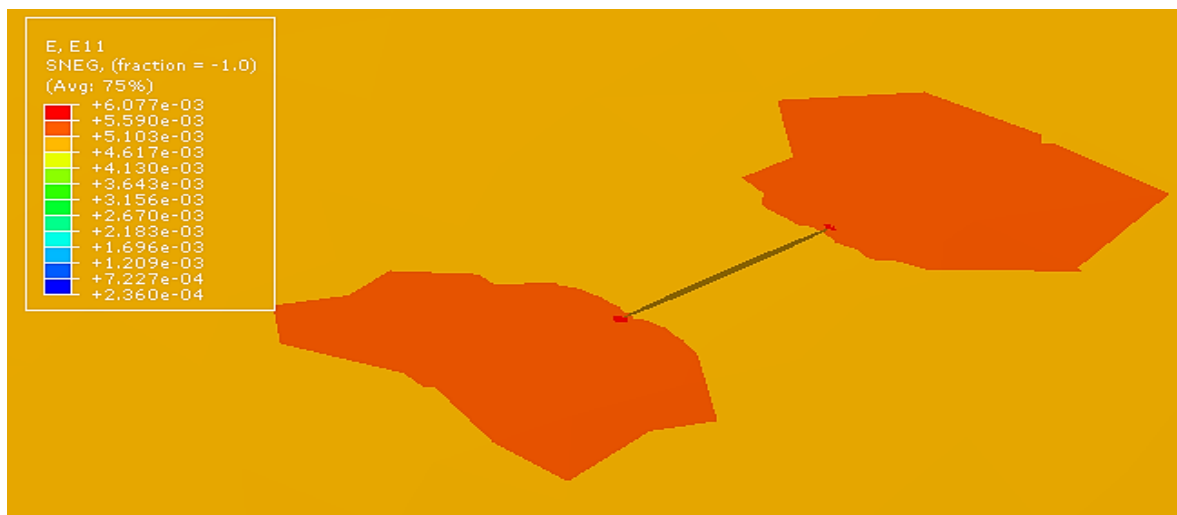
Figure 13: Strain at the crack tip under thermal stress.
