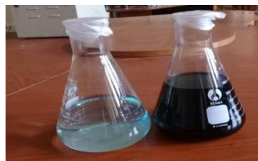
(B) Synthetic wastewater before and after treatment
