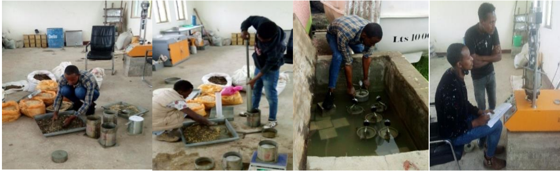
Figure 3.16 CBR and CBR Swell determination in Paragon Engineering Consultant PLC Laboratory
