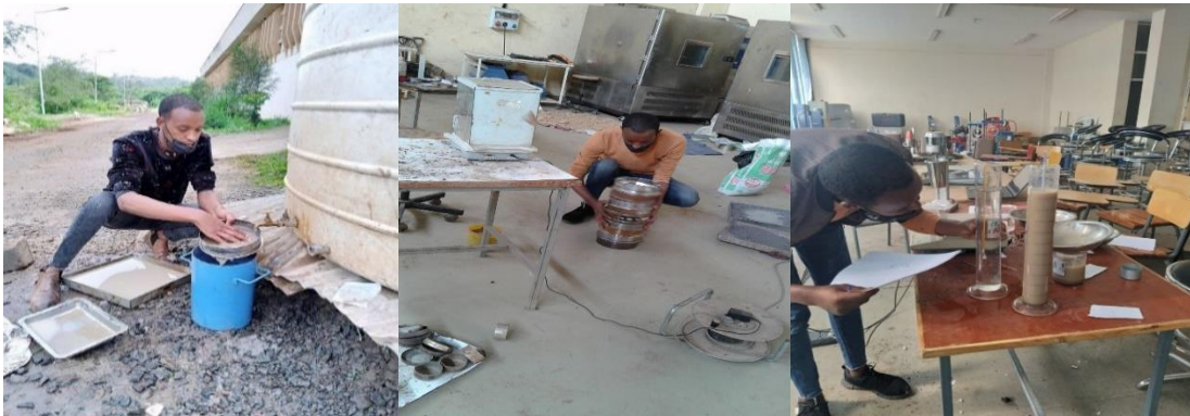
Figure 3.7 Grain size (Sieve and Hydrometer) test in JiT and MWU Geotechnical Engineering Laboratory
