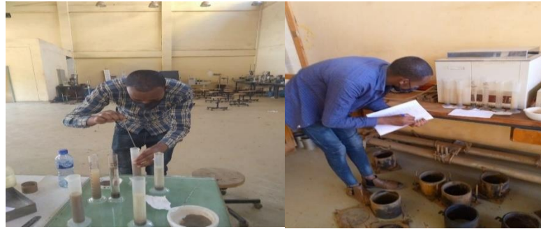
Figure 3.12 Free swell determination in JIT Geotechnical Engineering laboratory
