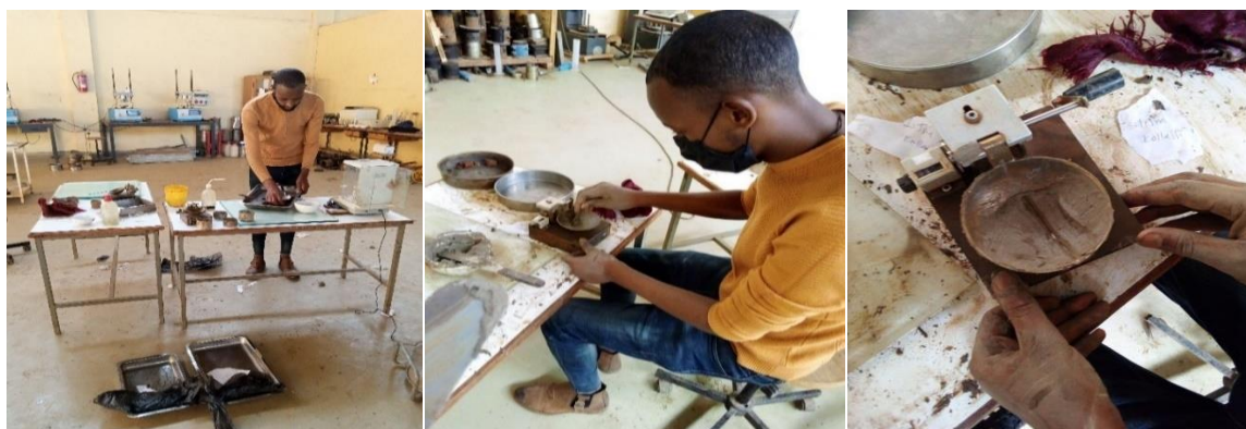
Figure 3.9 Liquid Limit determination in JIT Geotechnical Engineering laboratory
