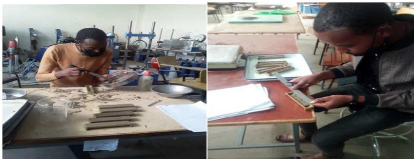
Figure 3.11 Linear shrinkage determination in MWU Civil Engineering Laboratory
