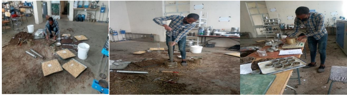
Figure 3.14 MDD and OMC determination in MWU Civil Engineering Laboratory
