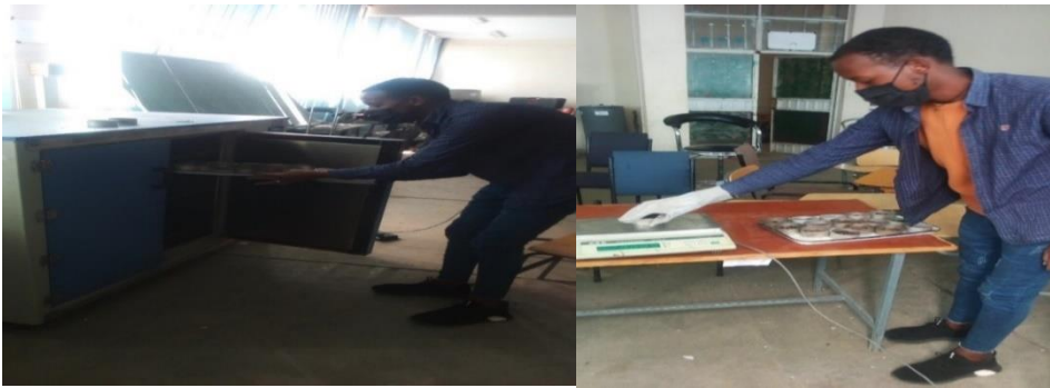
Figure 3.8 Natural moisture content determination in MWU Civil Engineering Laboratory
