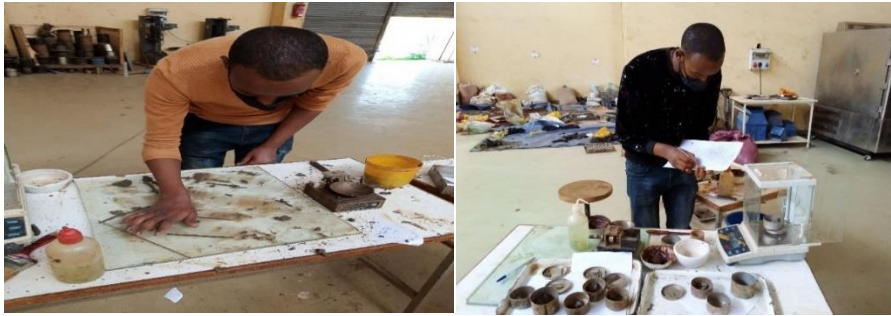
Figure 3.10 Plastic Limit determination in JIT Geotechnical Engineering laboratory
