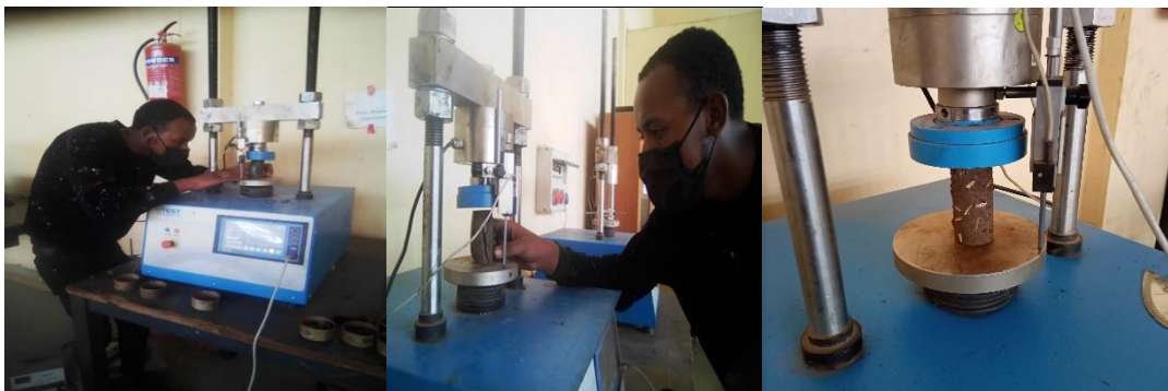
Figure 3.15 UCS determination in JIT Geotechnical Engineering laboratory
