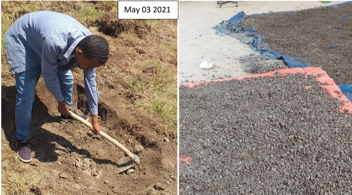
Figure 3. 2 Soil sample collection and preparation taken from my own phone
