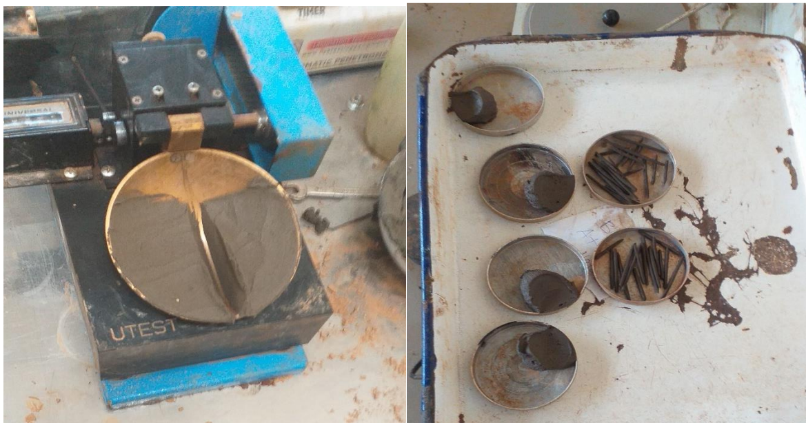
Figure 3. 7 Casagrande test taken from my own phone
