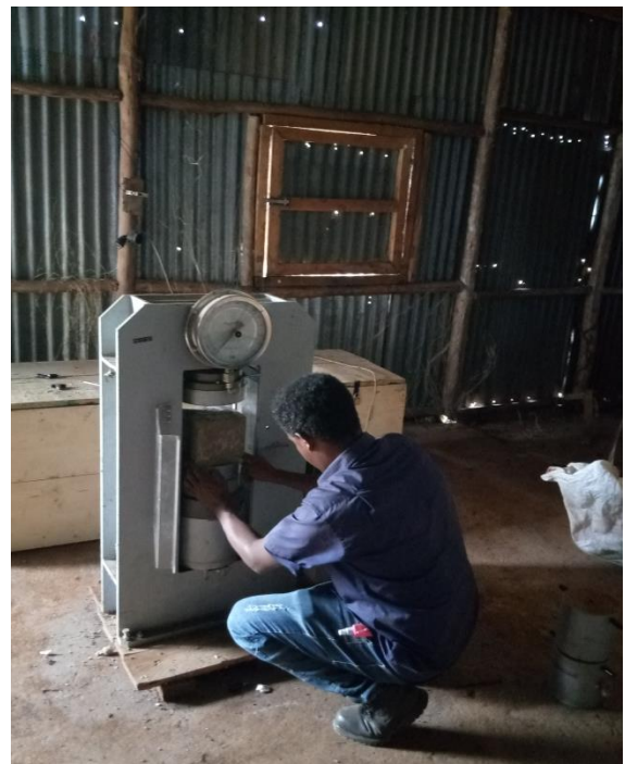
Figure F7: Putting Specimens on machine
