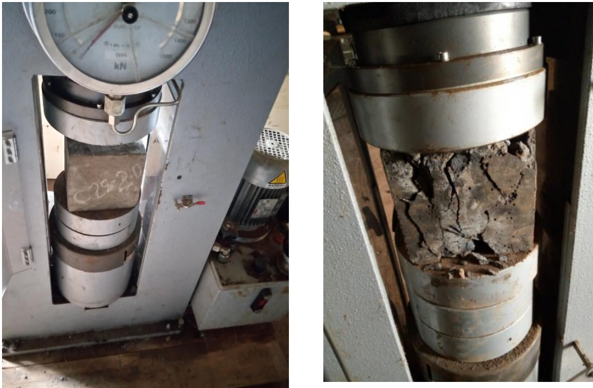
Figure 3.14: Compressive strength test set up and crushed specimen
