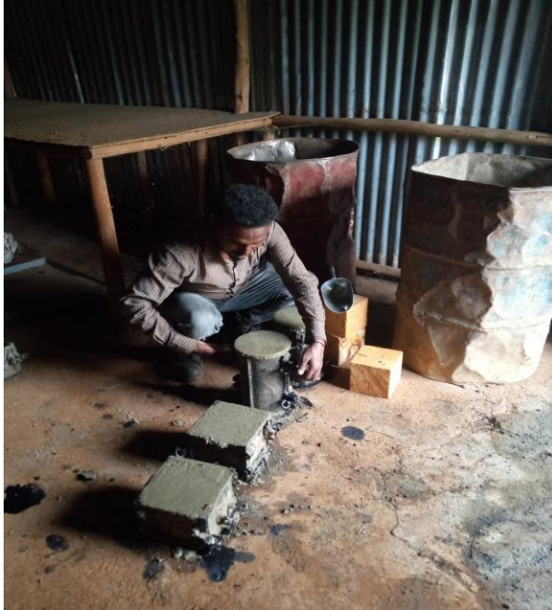
Figure F5: Casting RSFC Specimens
