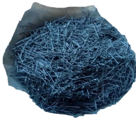
Figure 3.13: Preparation of recovered Steel fiber A) Recovered Bead wire from tire, B) Marking and cutting of recovered bead wire and C) Bead wire ready for mix.
