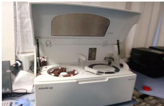
Figure 3.2: Mindray BS200E open, blood sample analysis machine on analysis samples
