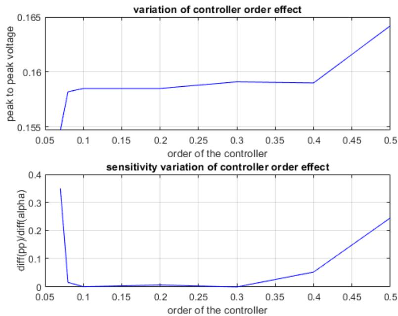
FIGURE 4.9: Relationship between Order of the Controller and Peak to Peak Output Voltage for FOSEPIC Converter (Boost Mode Operation)
