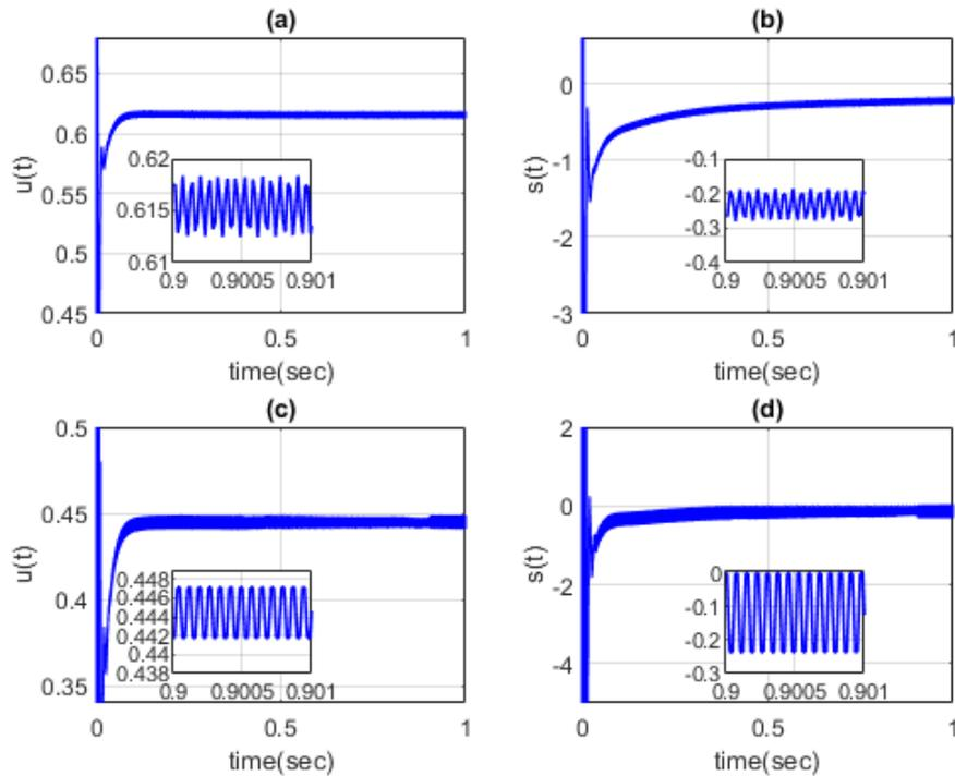
FIGURE 4.3: FOSEPIC Converter Sliding Surface and FOSMC
