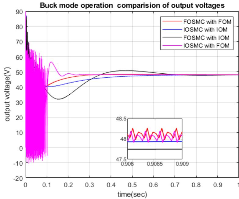
FIGURE 4.10: Comparison Output Voltage of SEPIC and FOSEPIC converter with FOMSC and IOSMC for Buck Mode Operation
