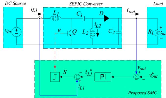
FIGURE 1.2: Overall Schematic Diagram of SEPIC Converter with SMC
