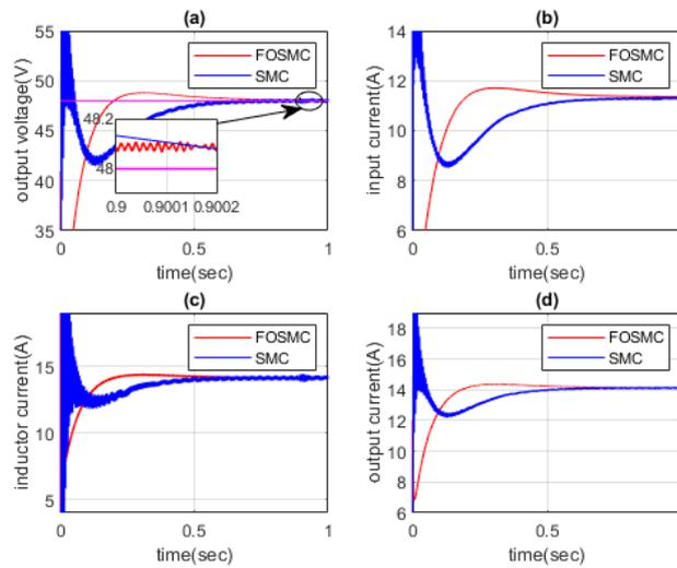
FIGURE 4.13: Comparison of Fractional and Integer SMC's for FOSEPIC Converter Under Buck Mode
