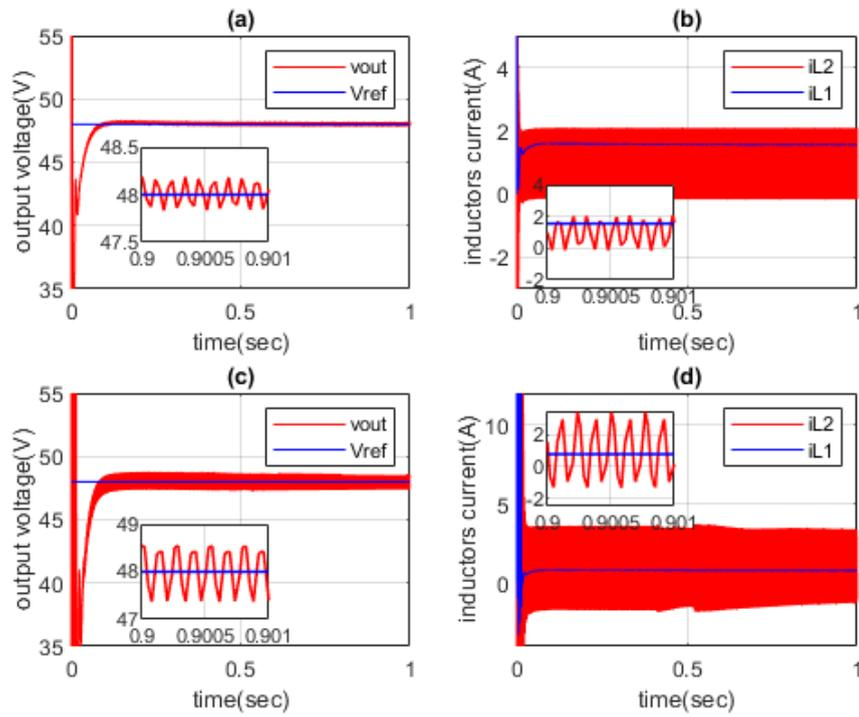
FIGURE 4.2: Steady-State Performance for FOSEPIC Converter
