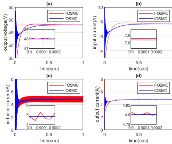
FIGURE 4.12: Comparison of Fractional and Integer SMC's for FOSEPIC Converter Under Boost Mode
