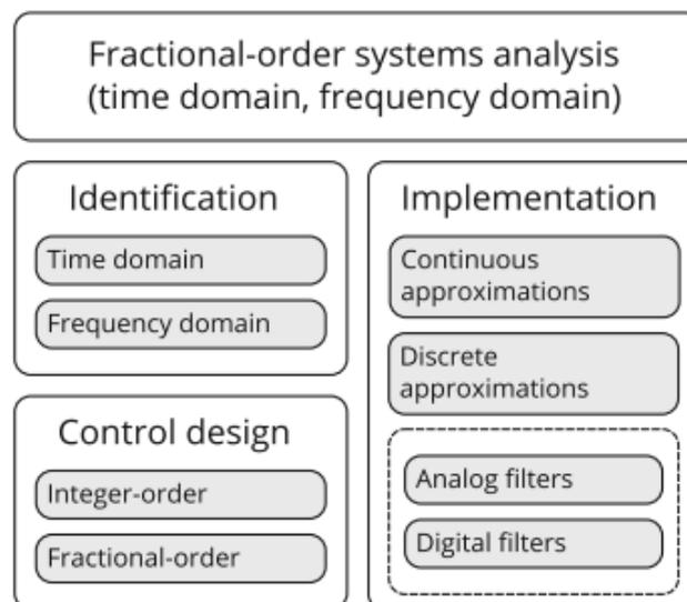
FIGURE 2.2: Modular Structure of the FOMCON Toolbox [31]
