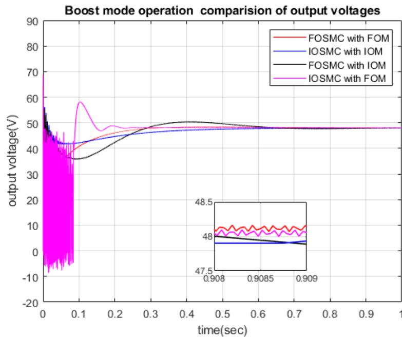
FIGURE 4.11: Comparison Output Voltage of SEPIC and FOSEPIC converter with FOMSC and IOSMC for Boost Mode Operation
