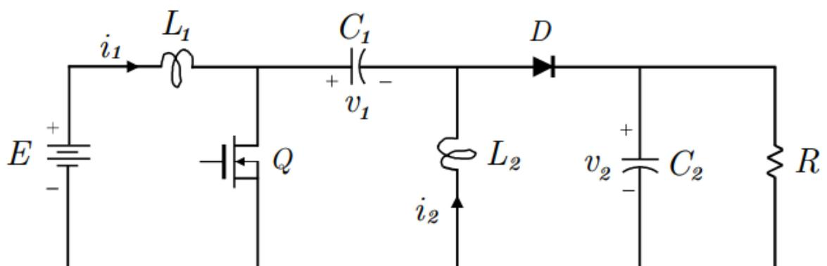
FIGURE 1.1: The SEPIC DC-to-DC Power Converter
