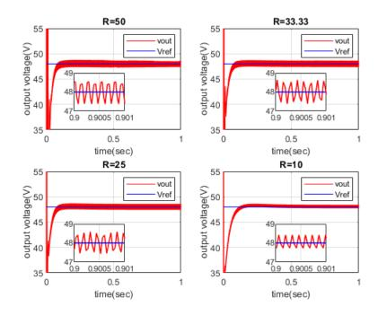
FIGURE 4.7: FOSEPIC Converter Under Load Variations for Buck Mode of Operation
