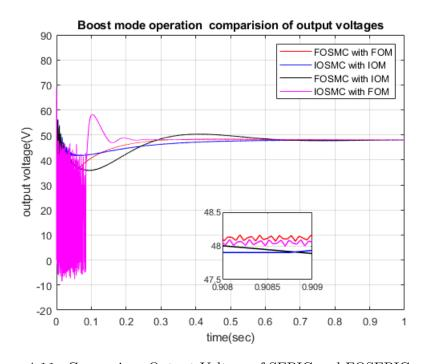
FIGURE 4.11: Comparison Output Voltage of SEPIC and FOSEPIC converter with FOMSC and IOSMC for Boost Mode Operation(a)[Red] FOSMC with FOM (b)[Blue] IOSMC with IOM(c)[Black] FOSMC with
