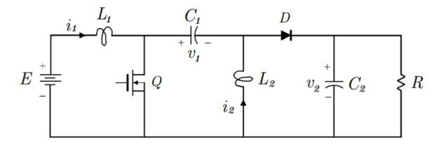
FIGURE 1.1: The SEPIC DC-to-DC Power Converter
