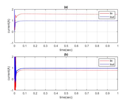
FIGURE 4.4: Input and Output Current for FOSEPIC Converter (a)Input and Output Current for Boost Mode of Operation (b) Input and Output Current for Buck Mode of Operation
