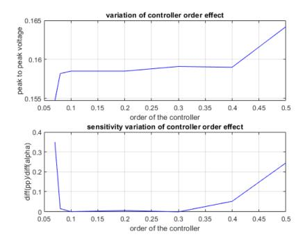
FIGURE 4.9: Relationship between Order of the Controller and Peak to Peak Output Voltage for FOSEPIC Converter (Boost Mode Operation)(a) Variation of Order Effect on Peak to Peak output Voltage (b)Sensitivity of the Variation of Order Effect on Peak to Peak output Voltage
