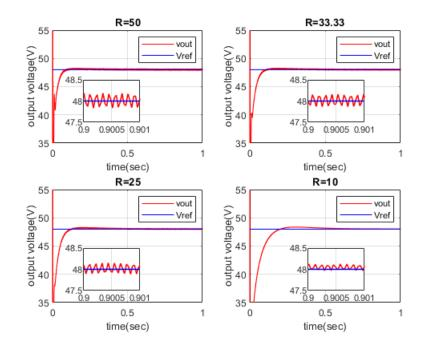
FIGURE 4.6: FOSEPIC Converter Under Load Variations for Boost Mode of Operation
