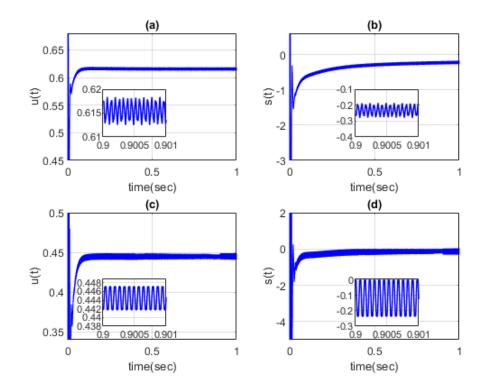
FIGURE 4.3: FOSEPIC Converter Sliding Surface and FOSMC (a)FOSMC for boost mode (b) Sliding surface for boost mode, (c)FOSMC for buck mode (d) sliding surface buck mode
