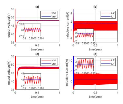
FIGURE 4.2: Steady-State Performance for FOSEPIC Converter (a) Output voltage for boost mode (c) Output voltage for buck mode, (b)Inductors current for boost mode (d) Inductors current buck mode
