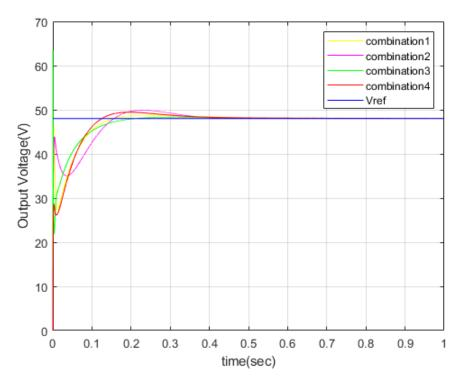
FIGURE 4.8: Output Voltage under Variation of FOSEPIC Orders (a)[Yellow] (0.6, 0.28, 0.4, 0.9) Combination1 (b)[Magenta] (0.9, 0.5, 0.4, 0.9) Combination2 (c)[Green] (0.17, 0.25, 0.35, 0.69) Combination3 (d)[Red] (0.75, 0.5, 0.2, 0.85) Combination4
