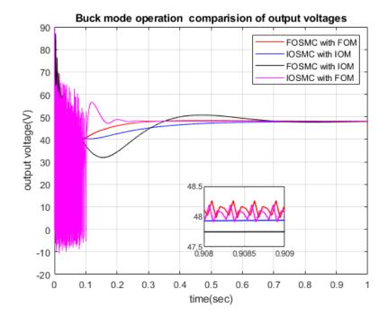
FIGURE 4.10: Comparison Output Voltage of SEPIC and FOSEPIC converter with FOMSC and IOSMC for Buck Mode Operation(a)[Red] FOSMC with FOM (b)[Blue] IOSMC with IOM(c)[Black] FOSMC with IOM (d)[Magenta] IOSMC with FOM
