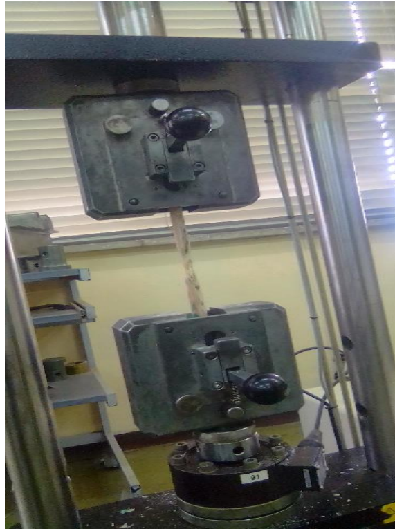
Figure 3.16 Specimen under tensile testing
