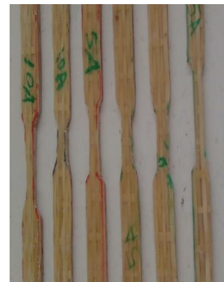
d) Laminated composite sample in mold e) Laminated bamboo epoxy composite mat f) ASTM, the standard of tensile specimen
