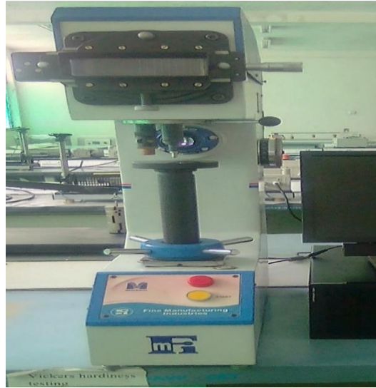
Figure 3.21 Vickers hardness test set up
