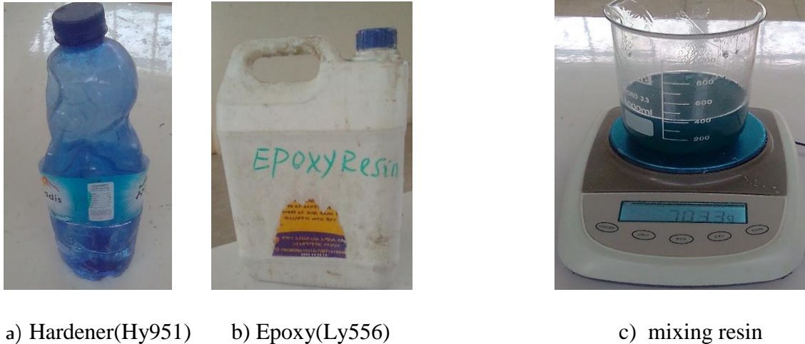
Figure 3.5 Epoxy and hardener resin mixed
