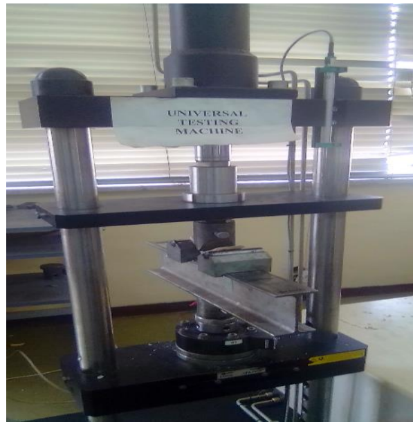
Figure 3.0.17 Specimen under flexural testing
