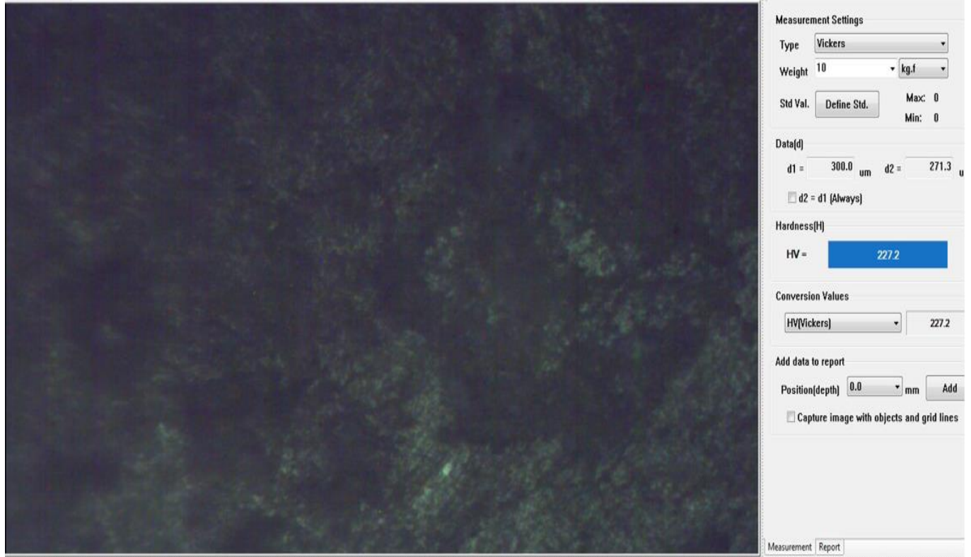
Vickers hardness test on \pm 45^{\circ} with the 10kgf
