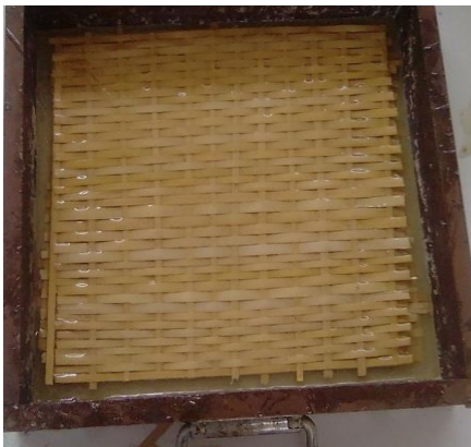
d) Laminated composite sample in mold e) Laminated bamboo epoxy composite mat f) ASTM, the standard of tensile specimen
