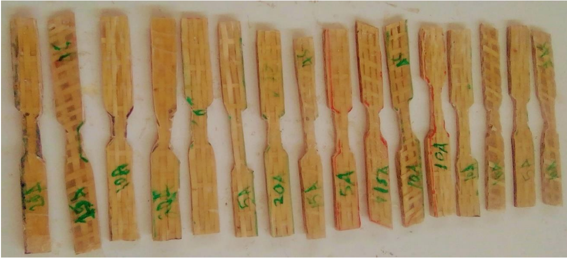
Figure 3.15 Tensile test sample
