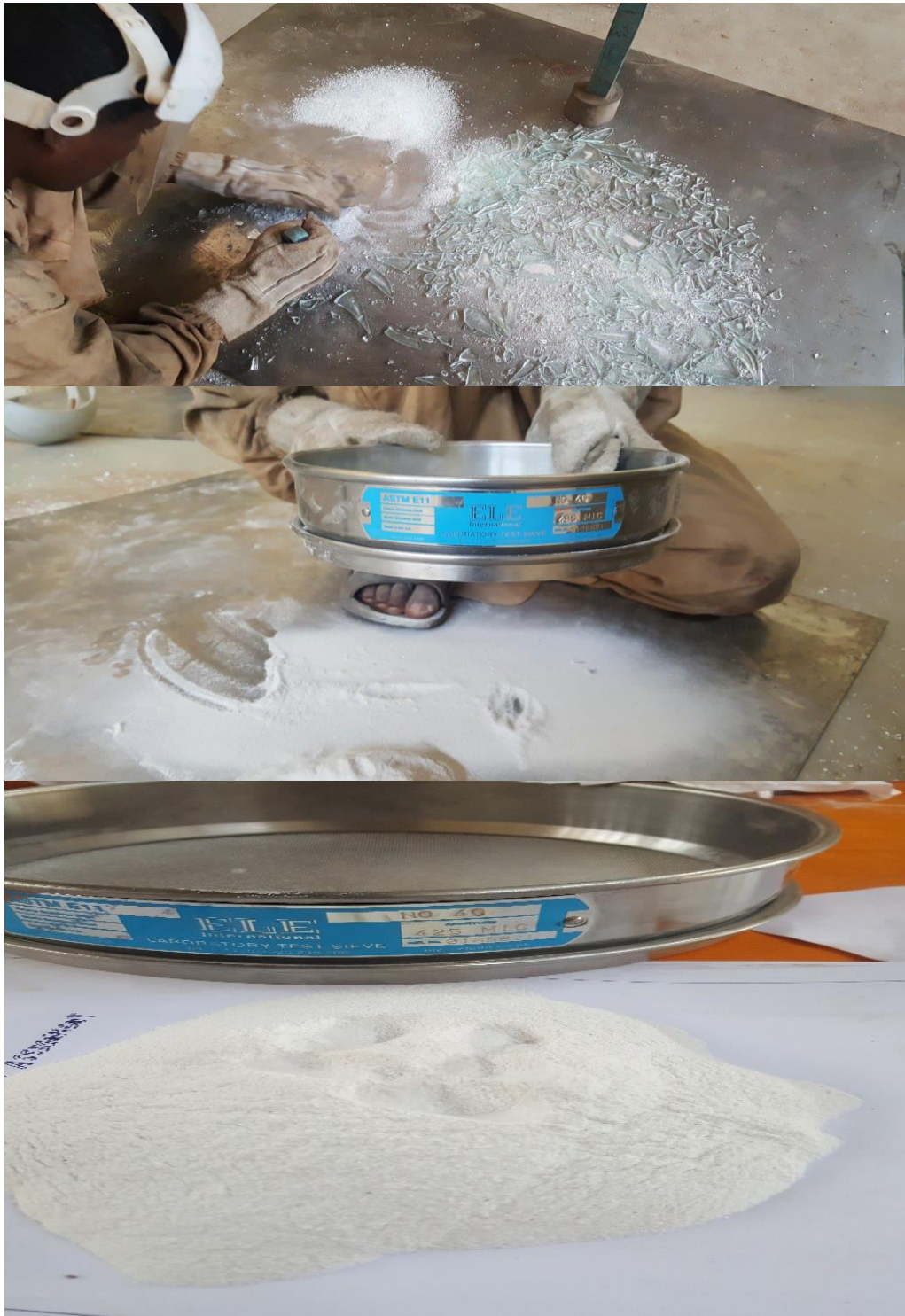
Figure 3.1 preparation reinforcement materials
