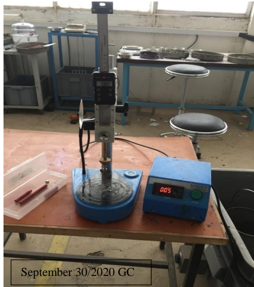
Figure3. 4 Digital bitumen penetration apparatus in Wolkite University
