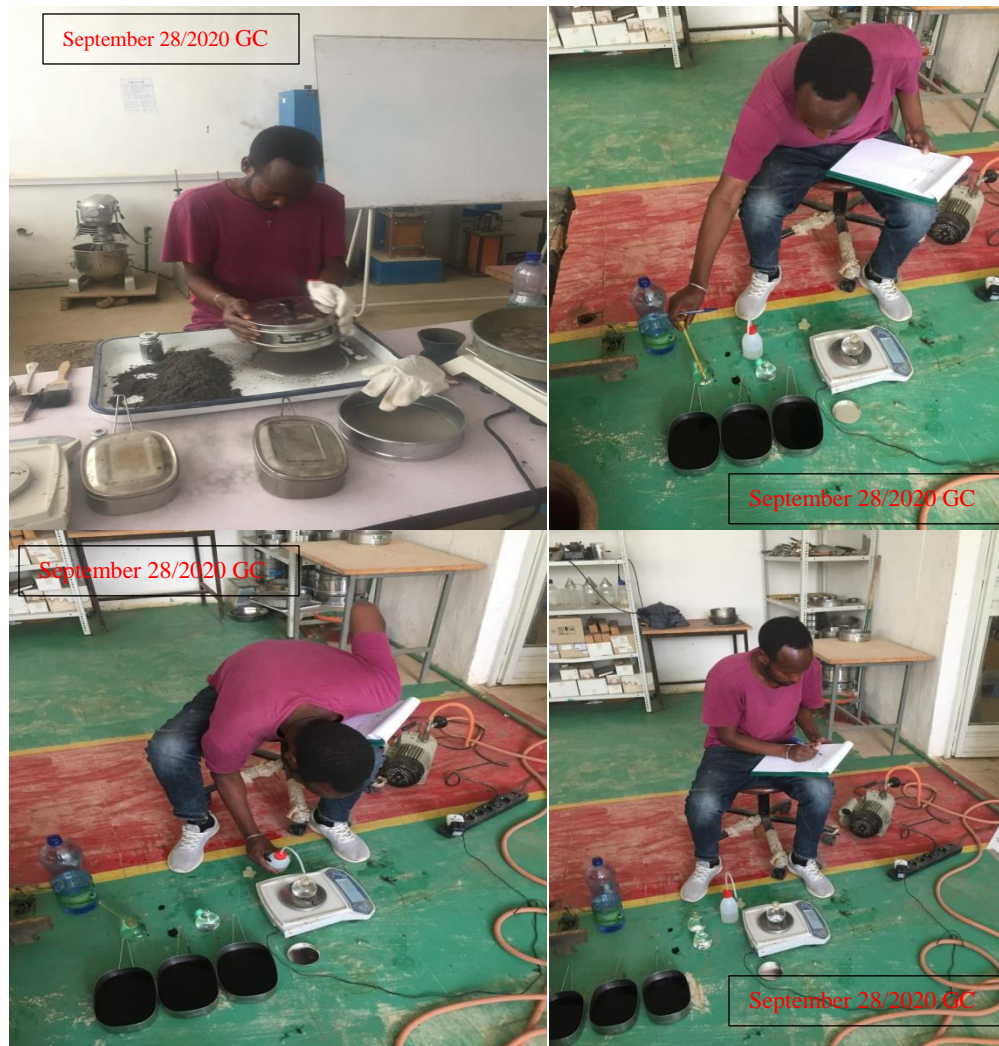
Figure3. 2 Determining specific gravity of filler material [Photo by Desta Moshe]
