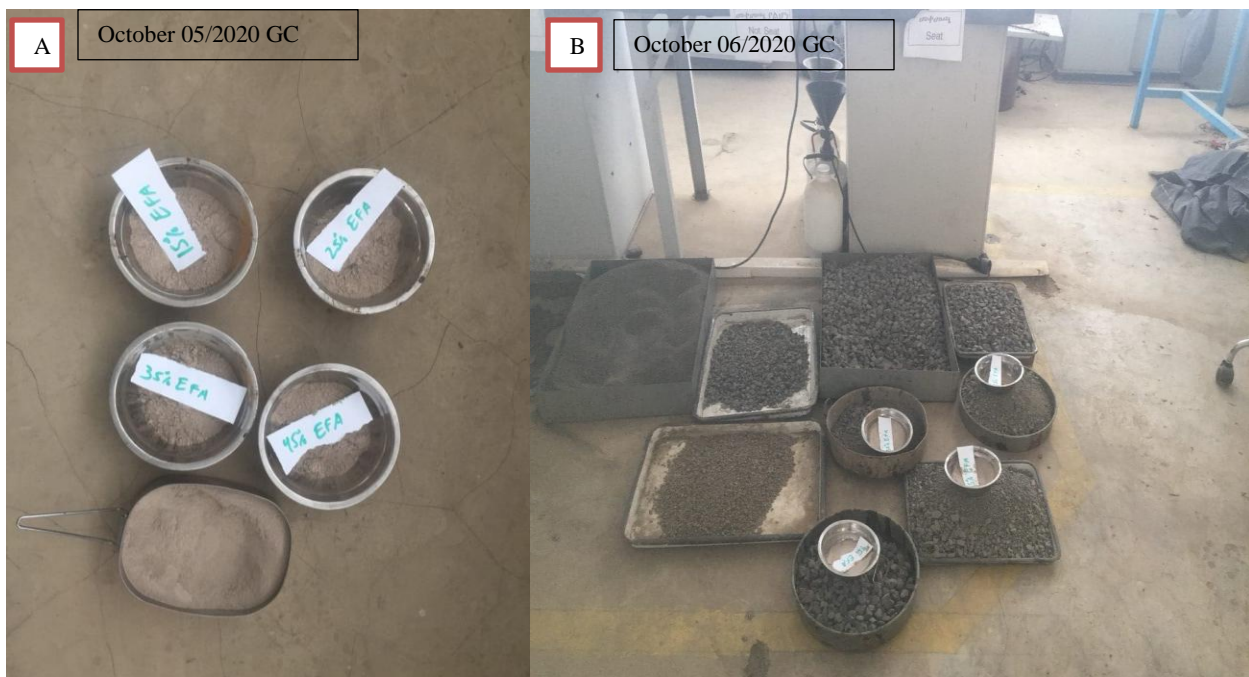
Figure3. 7 Aggregate preparation; A. EFA filler and B. Mixed aggregate
