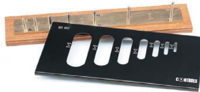
Figure3. 3 Flakiness and Elongation gages
