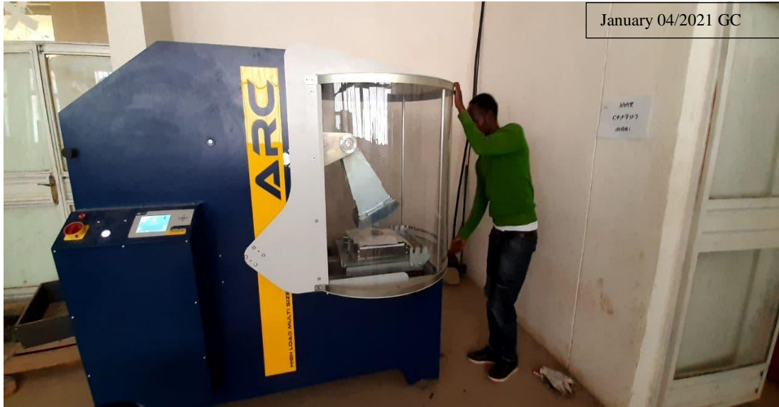
Figure3. 8 During ARC roller compactor operation for rutting specimen preparation
