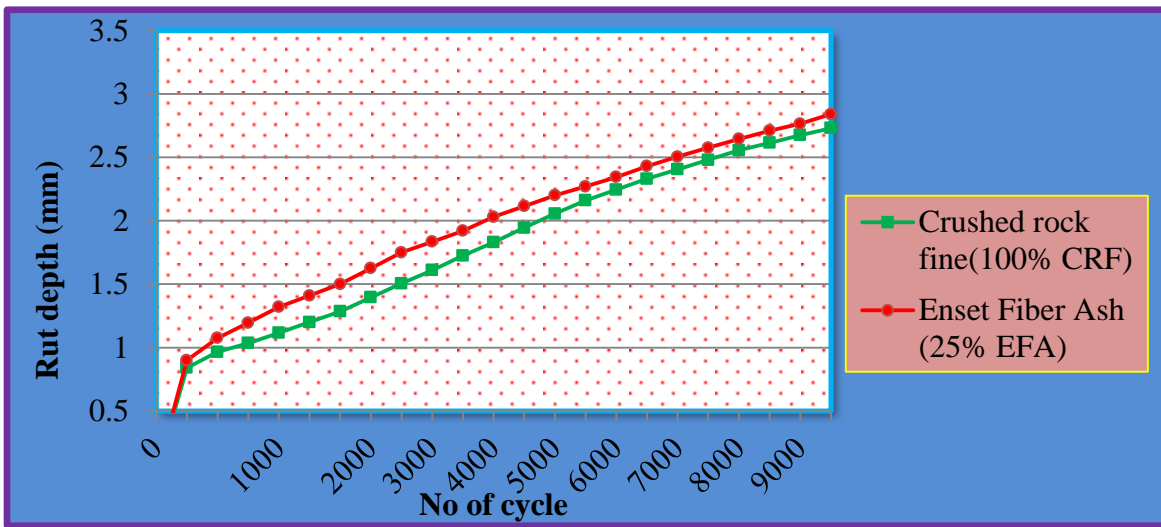
Figure4. 18: Wheel Tracking Test results for conventional and modified HMA
