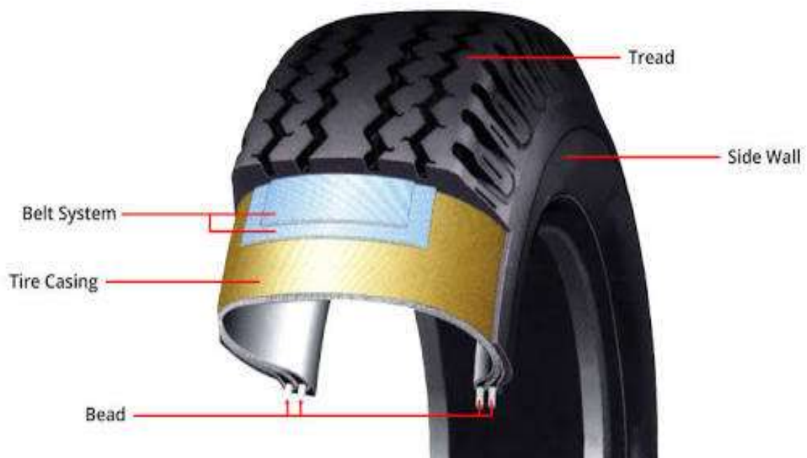
Figure 2.2: Tire structure, adapted from (Lo Presti., 2013).
