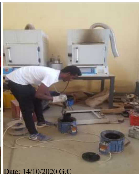
Source: Bilisumma Lemi Placing Bitumen on Heater
