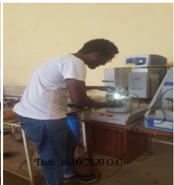
Source: Bilisumma Lemi Penetration of Bitumen
