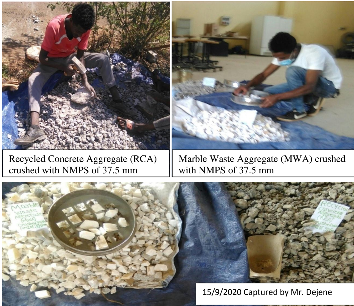
Figure 3.3 Sample of RCA and MWA crushed with NMPS of 37.5 - 0.075mm sieves
