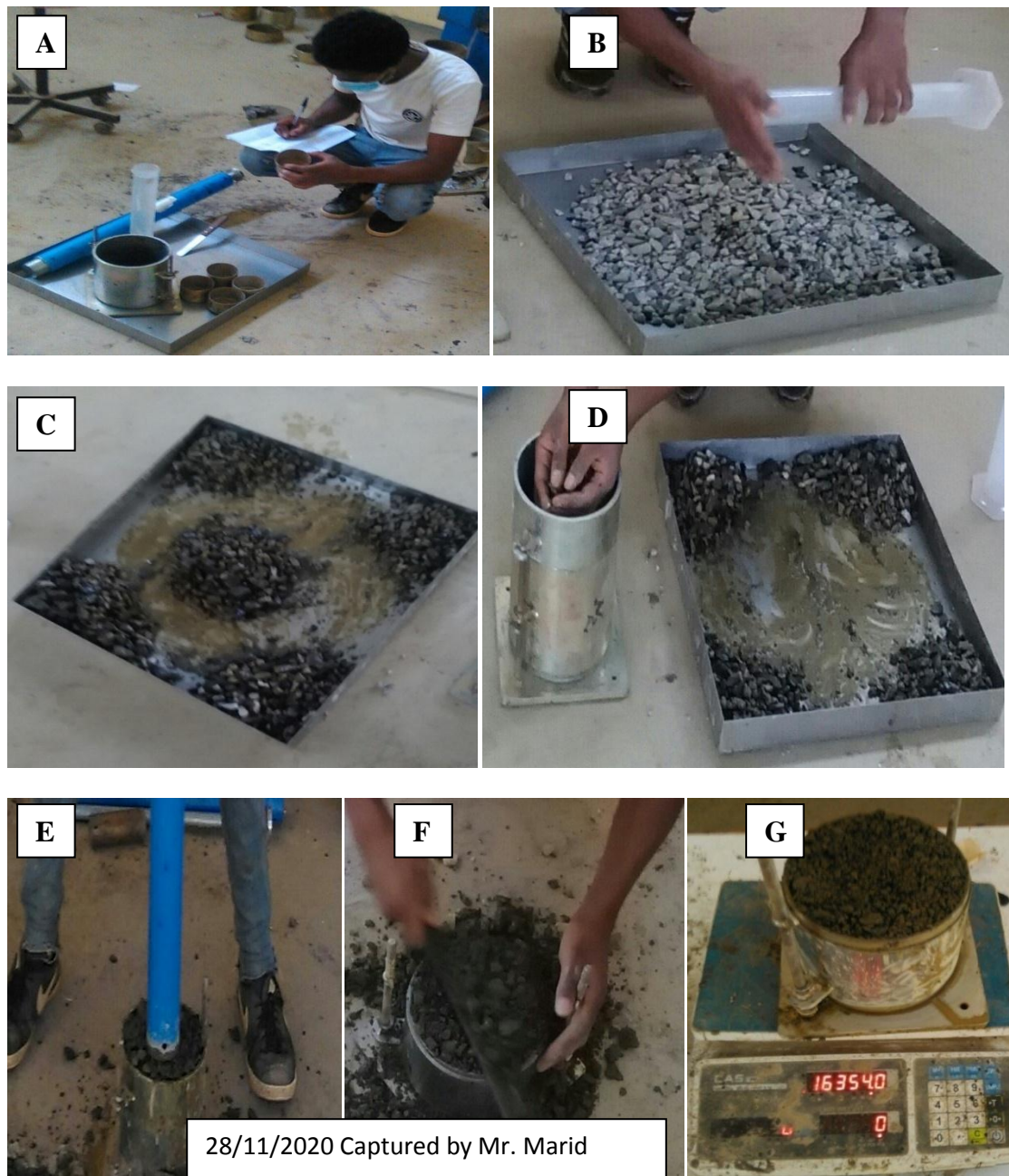
Figure 3.14 Typical compaction test procedures from (a) to (g)
