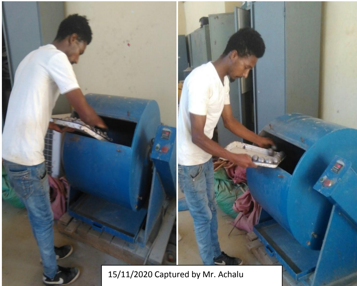
Figure 3.12 Drum machine and Abrasive charge balls used for Los Angeles Abrasion
