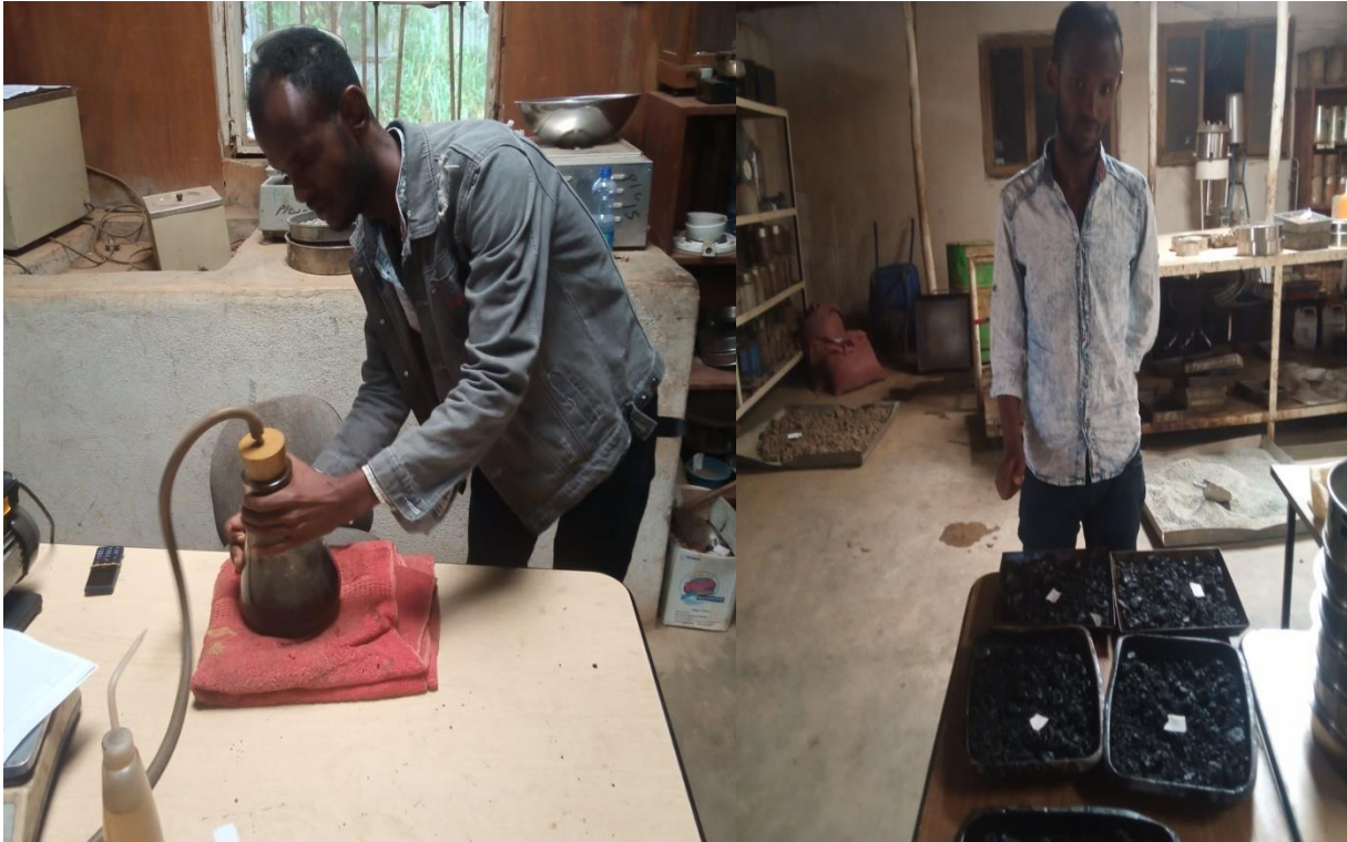
Figure 3.3.1 Theoretical Maximum Specific Gravity and Density determination
