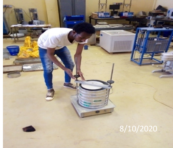
b) Aggregate sieve analysis
