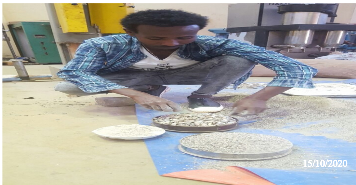
Figure 3. 3 Preparation of dust passing 0.075mm of CWP (Captured.by: Achalu Kebede)
