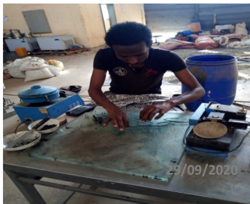
c) PI test for CHA
