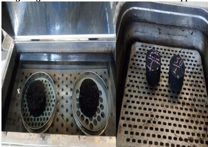
03/12/20, Captured by Kinfe G/georges Conditioned and UN conditioned specimen
