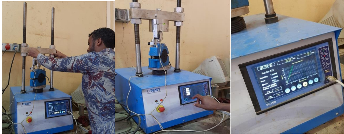
Fig. 3.15. Marshal Test apparatus seat up and (stability and flow) test in progress
