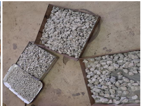
2/11/20, Captured by Mesganaw ayle quartering aggregates for test
