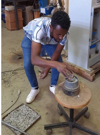
28/10/20, Captured by Dejeni Dreji Testing aggregates (ACV, AIV)
