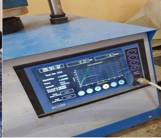
27/11/ 20, Captured by Dejni Dreji Marshal Stability and flow test in progress
