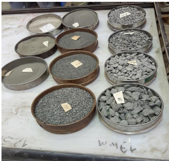
29/10/20, Captured by Kinfe G/G NCA for HMA preparation
