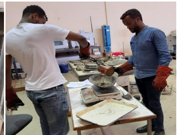
05/11/20, Captured by Hacalu Kebed Weighting aggregate and bitumen
