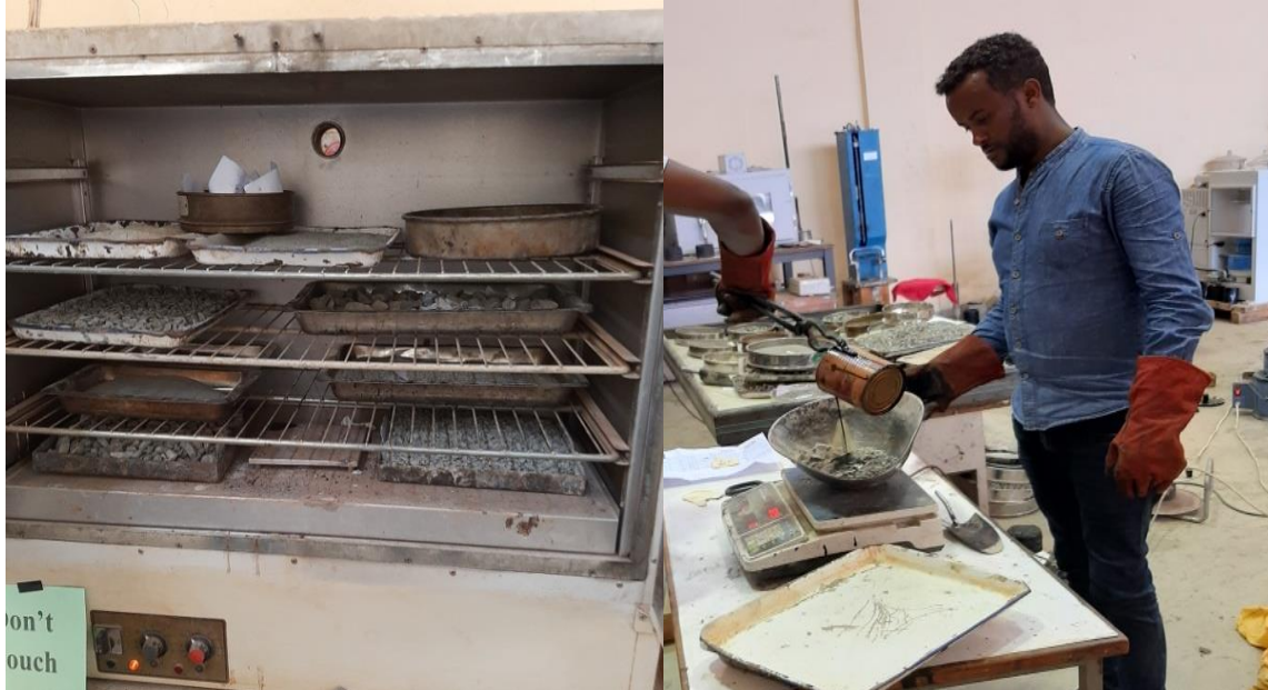
Fig. 3.11 Aggregates dried in oven and weighting of bitumen
