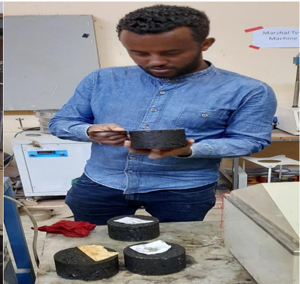
06/11/20, Captured by Hachalu Kebed weighting the spacemen for bulk specific gravity
