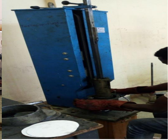
05/11/20, Captured by Kinfe G/g Compacting the mix 75 blows each side
