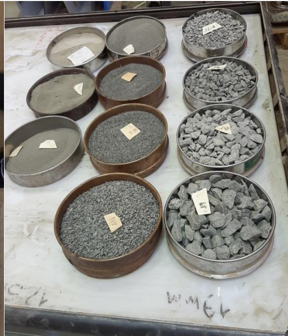
03/11/20, Captured by Kinfe G/georges Fig.3.7 Sieved aggregate (NCA)
