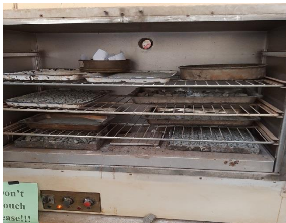
05/11/20, Captured by Kinfe G/G Aggregates in oven up to 24hr
