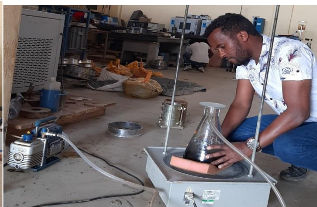
26/11/20, Captured by Dejni Dreji Vacuum application for saturated sample test
