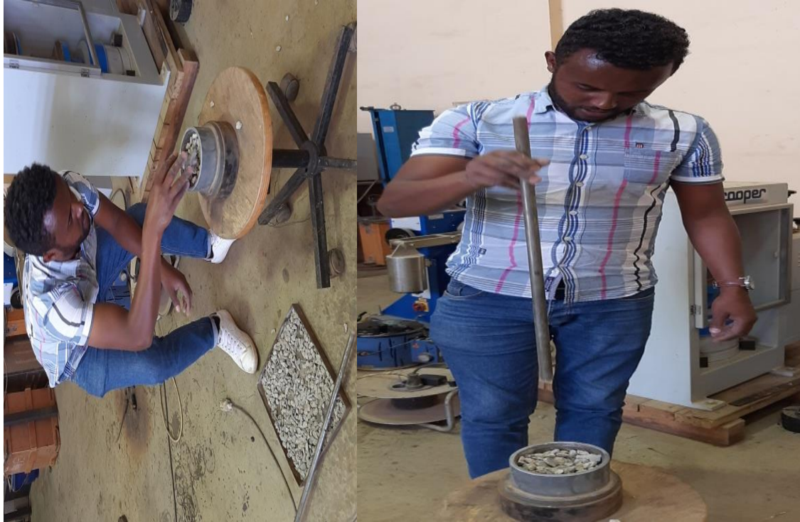
Fig.3.9 Aggregate crushing value (ACV) test for both DCWA &NCA
