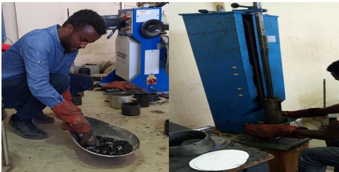
Fig - 3.12. Mixing of materials and compaction.
