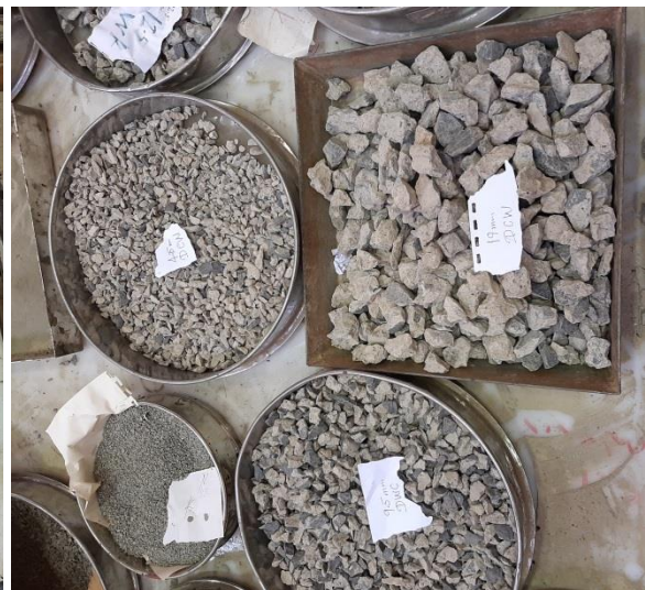
29/10/20, Captured by Kinfe.G/G DCWA for HMA preparation
