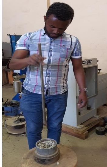
28/10/20, Captured by Dejeni Dreji Testing aggregates (ACV, AIV)
