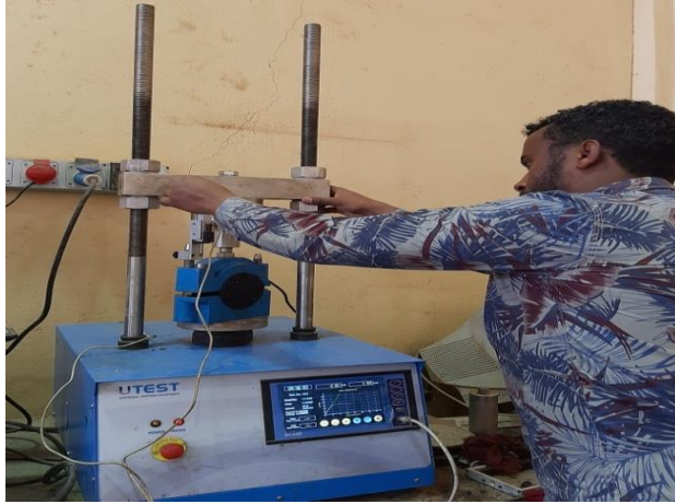
27/11/ 20, Captured by Dejni Dreji Marshal test apparatus seat up
