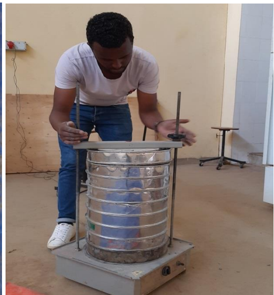
27/10/20, Captured by Mesganaw ayle Sieve the aggregates by standard sieve
