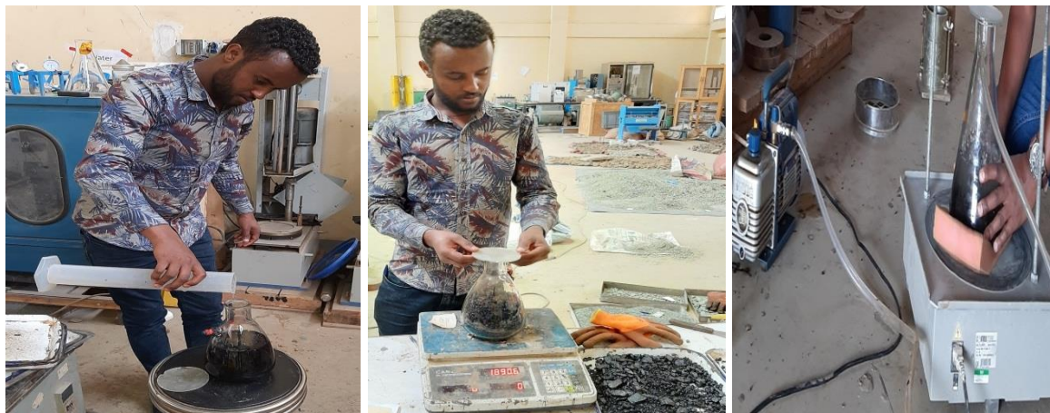
Fig. 3.16. Waighting los state mixture (a) and Vacuum application for saturated sample (b)
