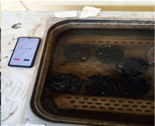
27/11/20, Captured by Kinfe.G/g Spacemen in water bath for 30minutes
