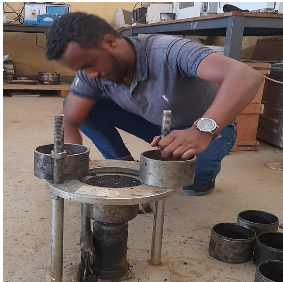
06/11/20, Captured by Hachalu Kebed Extruding spacemen after 24hr
