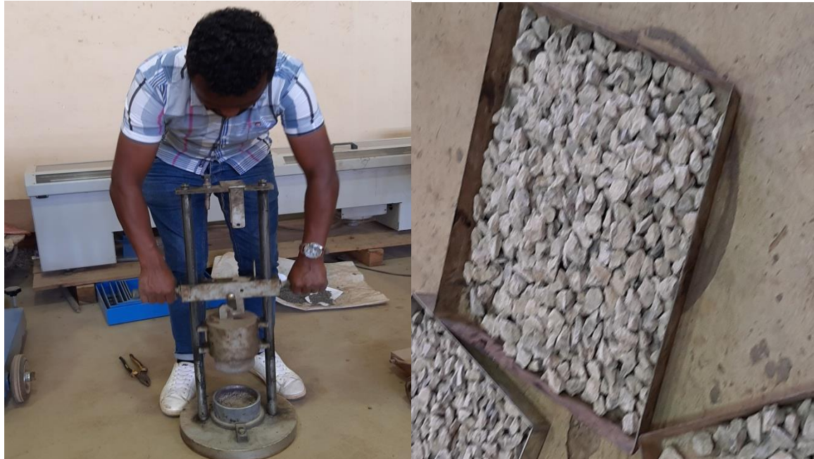
Fig .3.10.Aggregate Impact Test for both DCWA &NCA
