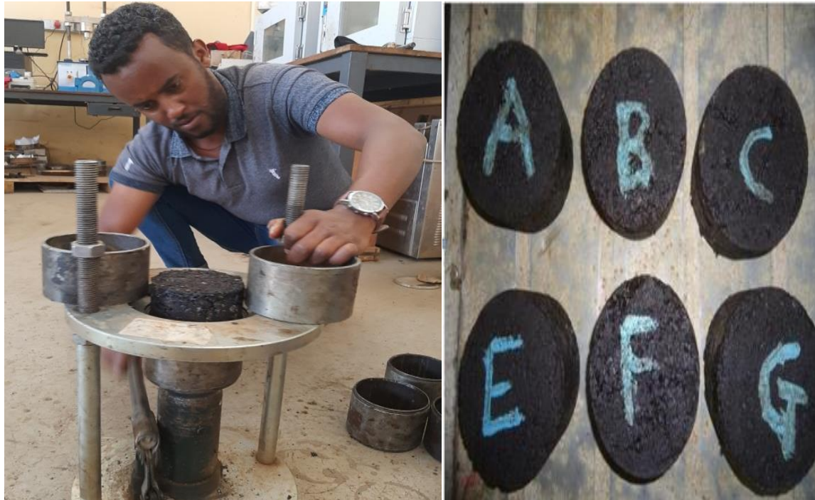
Fig. 3.13. Extrusion of compacted specimen after 24hr
