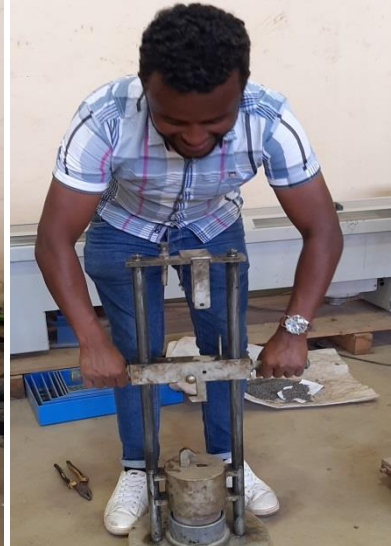
28/10/20, Captured by Dejeni Dreji Testing aggregates (ACV, AIV)
