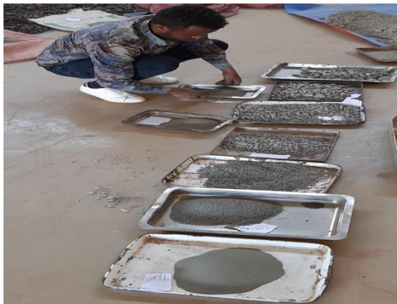
2/11/20, Captured by Mesganaw ayle Quartering aggregates for test
