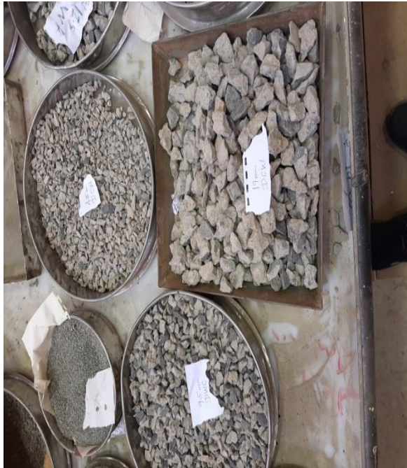
03/11/20, Captured by Kinfe G/georges Fig.3.6 Sieved aggregate (DCWA)
