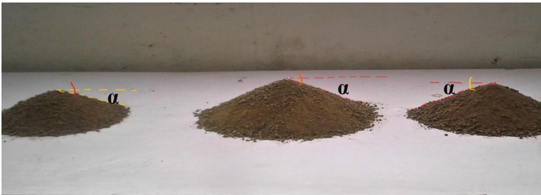
Figure 40. photo taken during determination of angle of repose in the laboratory.
